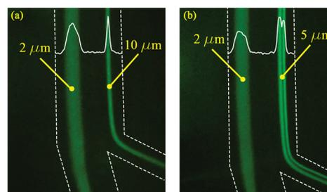
Fig. 5 The separation of 2  $\mu\text{m}$  particles from 10  $\mu\text{m}$  (a) at the flow rate of 1.0  $\text{mL min}^{-1}$ , and 2  $\mu\text{m}$  particles from 5  $\mu\text{m}$  (b) at the flow rate of 0.6  $\text{mL min}^{-1}$ .
