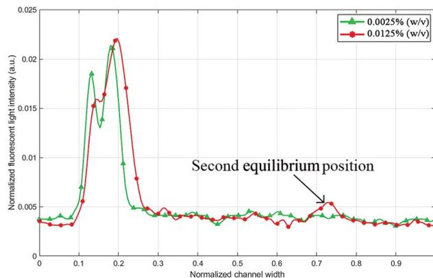
Fig. 3 Fluorescent green light intensity line profile (across the outlet channel) for 5  $\mu\text{m}$  particles with 0.0125% (w/v) and 0.0025% (w/v) suspension concentration at 0.7  $\text{mL min}^{-1}$ . Higher concentration values may increase the number of equilibrium positions.
