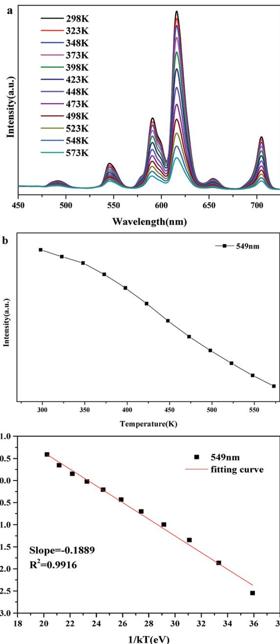
Fig. 12 (a) The luminescence spectra of  $\text{BLGOF}:0.15\text{Tb}^{3+}, 0.24\text{Eu}^{3+}$  at different temperatures (b) the intensity changes of  $\text{BLGOF}:0.15\text{Tb}^{3+}, 0.24\text{Eu}^{3+}$  phosphors 549 nm emission peak at different temperatures (c)  $\ln(I_0/I - 1)$  versus  $1/kT$  for the  $\text{BLGOF}:0.15\text{Tb}^{3+}, 0.24\text{Eu}^{3+}$ .
