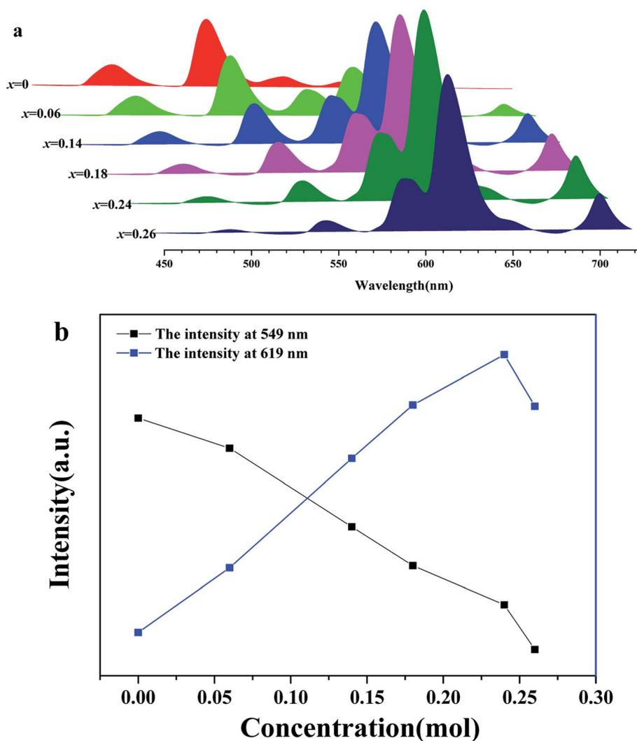
Fig. 6 (a) A series of luminescence spectra under 375 nm near-ultraviolet excitation of BLSOF:0.15Tb<sup>3+</sup>,*x*Eu<sup>3+</sup> ( $x = 0, 0.06, 0.14, 0.18, 0.24$  and  $0.26$ ) (b) the emission intensities of 549 nm (Tb<sup>3+</sup> characteristic emission spectra) and 619 nm (Eu<sup>3+</sup> characteristic emission spectra) at different Eu<sup>3+</sup> doping concentrations ( $x$ ) were measured under 375 nm excitation.
