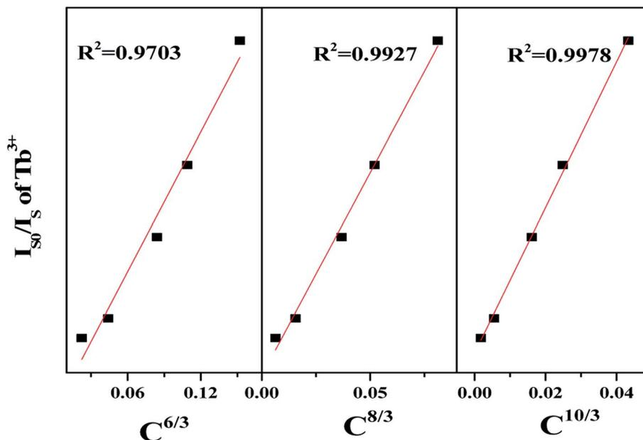
Fig. 9 The energy transfer mechanism from Tb<sup>3+</sup> to Eu<sup>3+</sup> of BLGOF:0.15Tb<sup>3+</sup>,xEu<sup>3+</sup> ( $x = 0.06, 0.14, 0.18, 0.24, \text{ and } 0.26$ ) phosphors.
