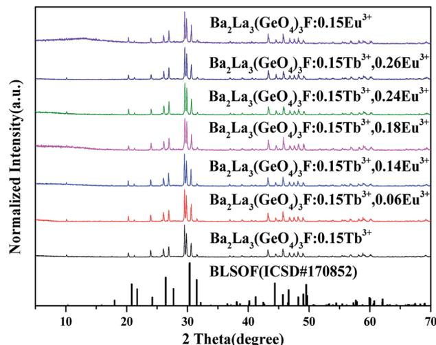
Fig. 1 XRD patterns of BLGOF:0.15Tb<sup>3+</sup>, BLGOF:0.15Eu<sup>3+</sup>, BLGOF:0.15Tb<sup>3+</sup>,xEu<sup>3+</sup> (x = 0.06, 0.14, 0.18, 0.24, and 0.26) phosphors, and standard data of BLSOF (ICSD#170852) is shown as a reference.
