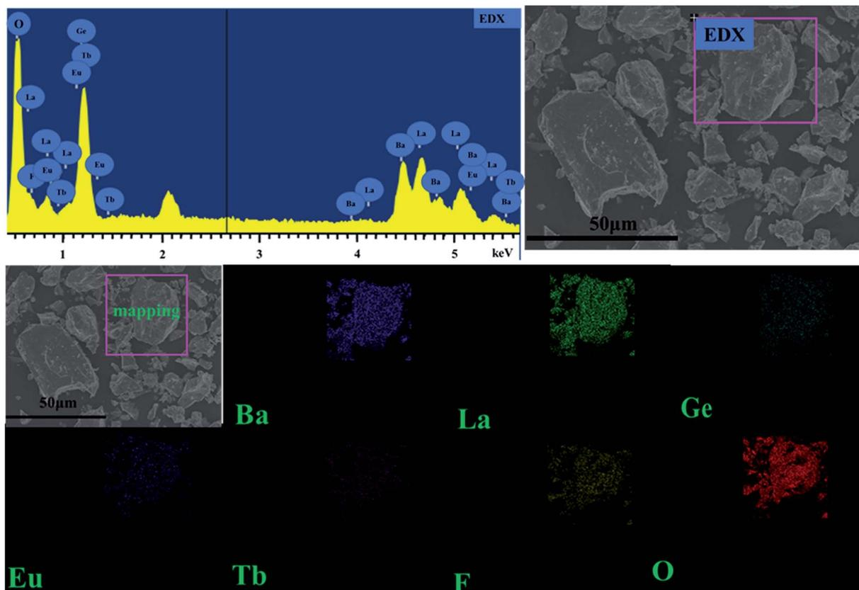
Fig. 3 (Top right) SEM image of BLGeOF:0.15Tb<sup>3+</sup>,0.15Eu<sup>3+</sup> phosphor (Top left) EDX spectra of BLGeOF:0.15Tb<sup>3+</sup>,0.15Eu<sup>3+</sup> phosphors (Bottom) elemental distribution of BLGeOF:0.15Tb<sup>3+</sup>,0.15Eu<sup>3+</sup> phosphors.
