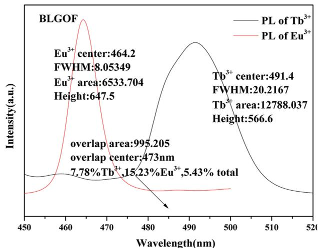
Fig. 5 Area integral and related parameters for the emission spectra of BLGeOF:0.15Tb<sup>3+</sup> phosphors, the excitation spectra of BLGeOF:0.15Eu<sup>3+</sup> phosphors and their overlapping parts.
