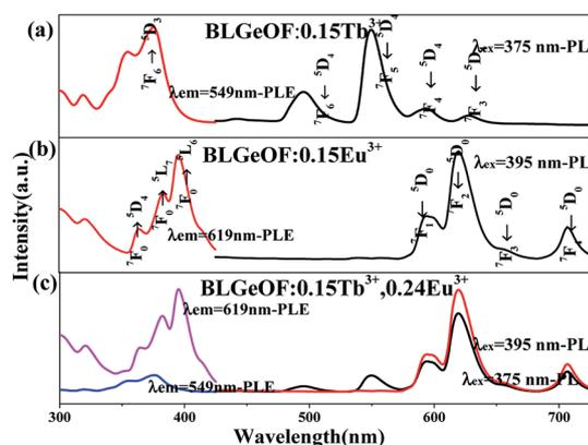
Fig. 4 (a) PLE spectrum (left) and PL spectrum (right) of BLGeOF:0.15Tb<sup>3+</sup> ( $\lambda_{em} = 549$  nm and  $\lambda_{ex} = 375$  nm) (b) PLE (left) and PL (right) spectra of BLGeOF:0.15Eu<sup>3+</sup> ( $\lambda_{em} = 619$  nm and  $\lambda_{ex} = 395$  nm) (c) PLE (left) and PL (right) spectra of BLGeOF:0.15Tb<sup>3+</sup>,0.24Eu<sup>3+</sup> ( $\lambda_{em} = 619$  nm and 549 nm;  $\lambda_{ex} = 375$ , and 395 nm).
