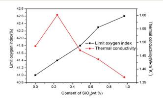
Fig. 7 LOI and thermal conductivity of  $SiO_2@Pb/B_4C/BPRs$  composites with different content of  $SiO_2$ .
