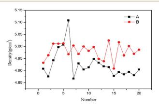
Fig. 6 Density of  $SiO_2@Pb/B_4C/BPRs$  composites in 20 regions. A: Pb/B<sub>4</sub>C/BPRs composites; B: 0.486 wt%  $SiO_2@Pb/B_4C/BPRs$  composites.
