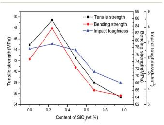
Fig. 9 Mechanical properties of SiO<sub>2</sub>@Pb/B<sub>4</sub>C/BPRs composites with different content of SiO<sub>2</sub>
