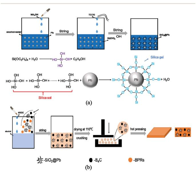
Fig. 1 (a) Schematic diagram of the synthesis of  $SiO_2$ @Pb powders; (b) schematic diagram of the preparation of  $SiO_2$ @Pb/B<sub>4</sub>C/BPRs composites.
