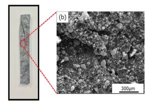
Fig. 8 Photographs and SEM images of SiO<sub>2</sub>@Pb/B<sub>4</sub>C/BPRs composites after burning with different content of SiO<sub>2</sub>: (a) Pb, (b) 0.486 wt% SiO2@Pb, (c) 0.967 wt% SiO2@Pb.
