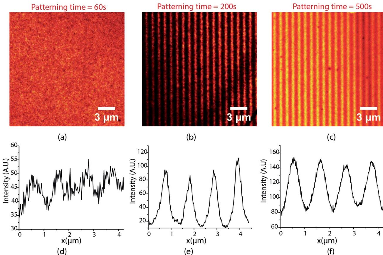
Fig. 4 STED images for patterns fabricated with  $80 \text{ mW cm}^{-2}$  excitation intensity and  $85 \text{ W cm}^{-2}$  depletion intensity using 1 micron green standing wave periodicity exposed for (a) 60 seconds (b) 200 seconds (c) 500 seconds. Line profiles for the lines show in (d) for (a), (e) for (b) and (f) for (c).
