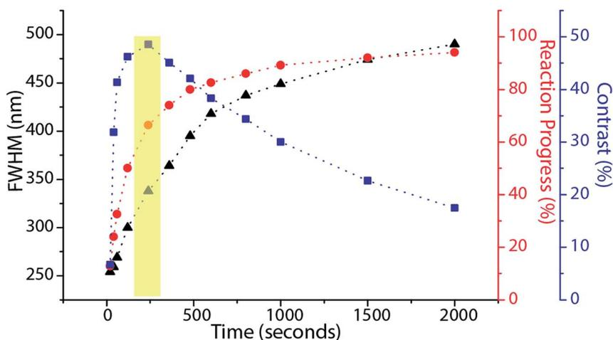
Fig. 6 The calculated FWHM, Michael addition yield and line contrast as a function of time for  $80 \text{ mW cm}^{-2}$  excitation intensity and  $85 \text{ W cm}^{-2}$  depletion intensity with 1 micron green standing wave periodicity. The optimal exposure window for high contrast patterning is shaded in yellow.
