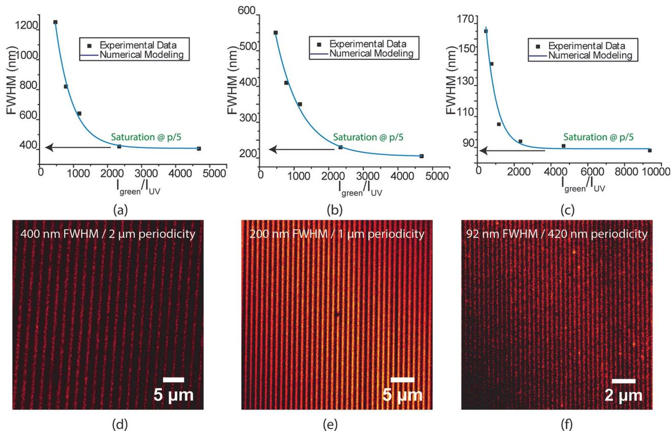
Fig. 3 Plot of linewidth as a function of green to UV intensity ratio for (a) 2 micron (b) 1 micron and (c) 420 nm green standing wave periodicity. STED images for patterns fabricated with  $40 \text{ mW cm}^{-2}$  excitation intensity and  $190 \text{ W cm}^{-2}$  depletion intensity using (d) 2 micron (e) 1 micron and (f) 420 nm green standing wave periodicity.
