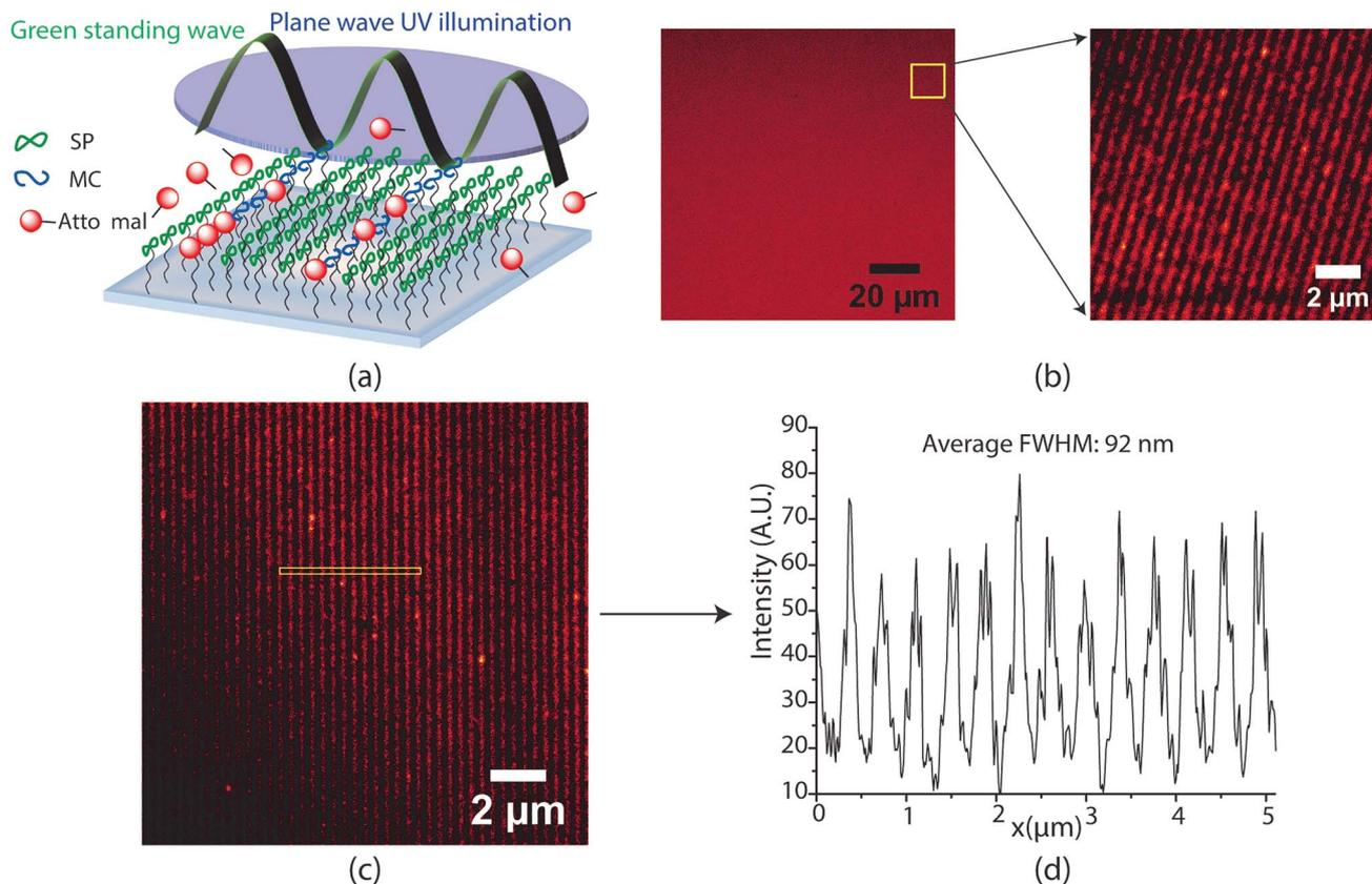
Fig. 2 (a) Super-resolution interference lithography scheme using spirothiopyran monolayers. (b) 50  $\mu\text{m}$  and zoomed 10  $\mu\text{m}$  inset frame showing confocal microscopy images of patterned lines obtained. (c) STED microscope image of lines fabricated using a 420 nm period depletion (green) standing wave. (d) Line profiles for (c). The average FWHM was found to be 92 nm.
