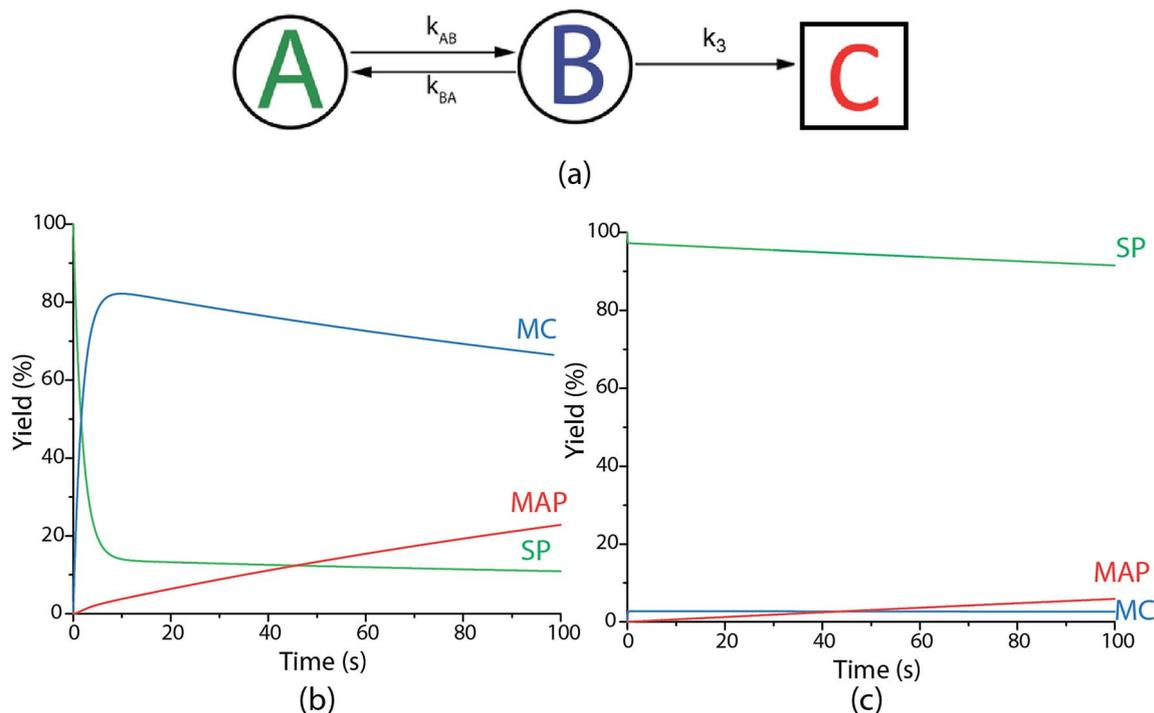
Fig. 5 (a) Schematic used to construct the numerical photokinetic model for the spirothiopyran writing system. Modelling is performed for a constant (plane wave) excitation and sinusoidal (periodic) depletion intensity profiles. The change in concentration of the various chemical species involved as function of time is plotted for the (b) minima and (c) maxima of the depletion beam.
