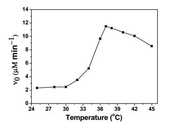
Fig. 7 The catalytic rate of PNTegel as a function of temperature for the catalytic reduction of CUOOH (0.25 mM) by TNB (0.15 mM) with a catalytic center of 1.00 µM.
