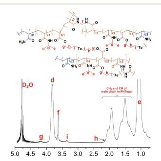
Fig. 2 <sup>1</sup>H NMR spectrum of PNTegel in D<sub>2</sub>O.
