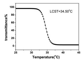
Fig. 5 Temperature dependences of optical transmittance at 600 nm obtained for PNTegel at the concentration of 1 mg mL<sup>-1</sup>
