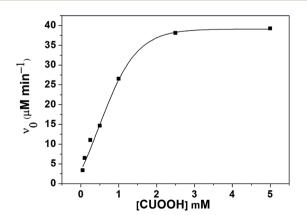
Fig. 9 The catalytic rate as a function of concentration of CUOOH in the presence of the **PNTegel**. The initial concentration of TNB was fixed to be 0.15 mM, the concentration of CUOOH was 0.05, 0.10, 0.25, 0.5, 1, 2.5 and 5 mM, respectively.
