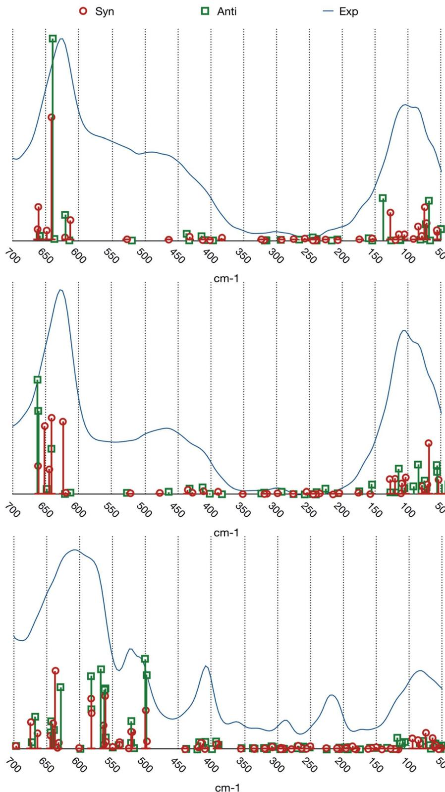
Fig. 3 Comparison between the experimental spectra and calculated normal modes frequencies and intensities. From top to bottom:  $[\text{BIC}_4\text{IB}]^{2+} + 2\text{Br}^-$ ,  $[\text{BIC}_5\text{IB}]^{2+} + 2\text{Br}^-$  and  $[\text{MIC}_6\text{IM}]^{2+} + 2\text{Tf}_2\text{N}^-$ .
