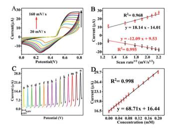
Fig. 3 (A) CVs of the Ni-MOF/Nafion/GCE electrode with 1.0 mM urea at distinct scan speeds: 20, 40, 60, 80, 100, 120, 140, 160 mV s<sup>-1</sup>. (B) The plot of variation of anode and cathode peak currents with scanning rate. (C) DPV of the Ni-MOF/Nafion/GCE electrode at variant urea concentrations: 0-0.2 mM. Test factors: amplitude 0.05 V, pulse cycle time 0.2 s and impulse duration 0.05 s. (D) The correlation of associated response vs. the concentration.
