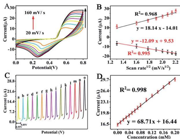
Fig. 3 (A) CVs of the Ni-MOF/Nafion/GCE electrode with 1.0 mM urea at distinct scan speeds: 20, 40, 60, 80, 100, 120, 140, 160 mV s<sup>-1</sup>. (B) The plot of variation of anode and cathode peak currents with scanning rate. (C) DPV of the Ni-MOF/Nafion/GCE electrode at variant urea concentrations: 0–0.2 mM. Test factors: amplitude 0.05 V, pulse cycle time 0.2 s and impulse duration 0.05 s. (D) The correlation of associated response vs. the concentration.
