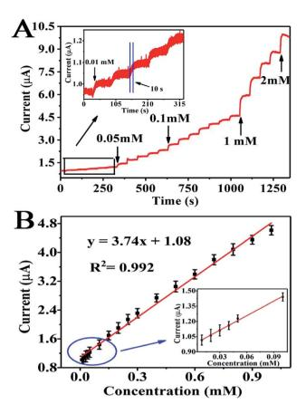
Fig. 5 (A) Amperometric i-t curve for unceasing additions of urea into the electrolyte solution at oxidation peak potential of +0.6 V. (B) The calibration curve is shown about  $I_{pa}$  ( $\mu$ A) and C (mM).
