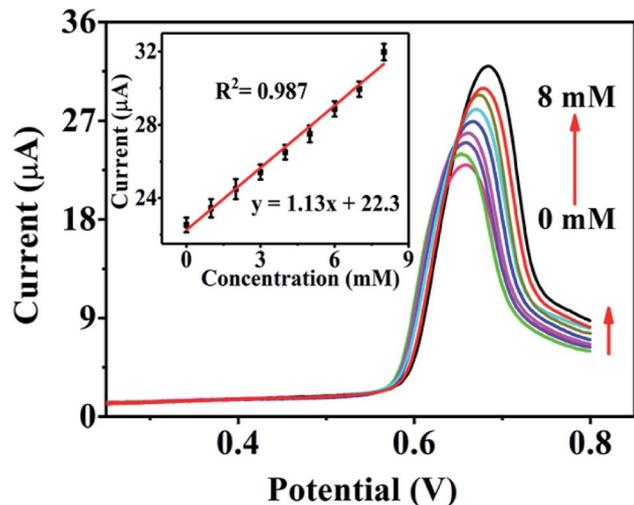
Fig. 7 LSV responses of Ni-MOF nanobelts modified GCE in diluted human urine sample containing different urea concentrations: 0, 1, 2, 3, 4, 5, 6, 7, and 8 mM. Inset: Corresponding calibration plot of urea concentration vs. current response.
