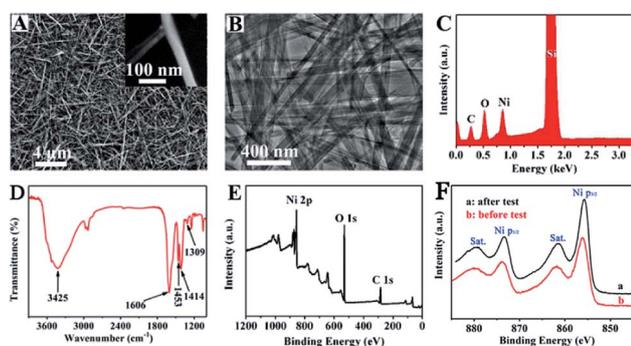
Fig. 1 Low (A) and high (the inset) magnification SEM images of Ni-MOFs; (B) TEM image of Ni-MOFs; (C) EDX spectrum of Ni-MOFs; (D) FT-IR spectrum of Ni-MOFs; XPS patterns of survey (E) and Ni  $2p$  regions before and after testing (F) on the Ni-MOFs.
