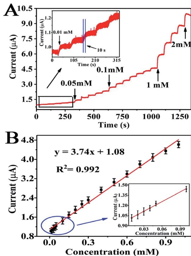
Fig. 5 (A) Amperometric  $i-t$  curve for unceasing additions of urea into the electrolyte solution at oxidation peak potential of +0.6 V. (B) The calibration curve is shown about  $I_{pa}$  ( $\mu\text{A}$ ) and  $C$  (mM).
