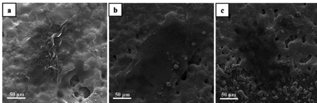
Fig. 2 Typical SEM images of (a) rGO, (b) 4HQ-rGO and (c) 4HQ-rGO/Cu<sup>2+</sup> deposited on the surface of IDEs used for acetic acid gas sensing.
