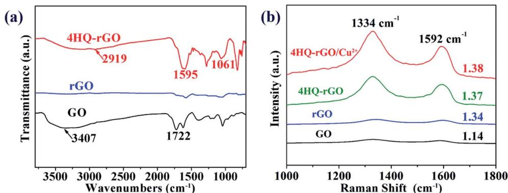
Fig. 3 (a) FT-IR spectra of the GO, rGO, and 4HQ-rGO material. (b) Raman spectra of the GO, rGO, 4HQ-rGO, and 4HQ-rGO/Cu<sup>2+</sup> material.
