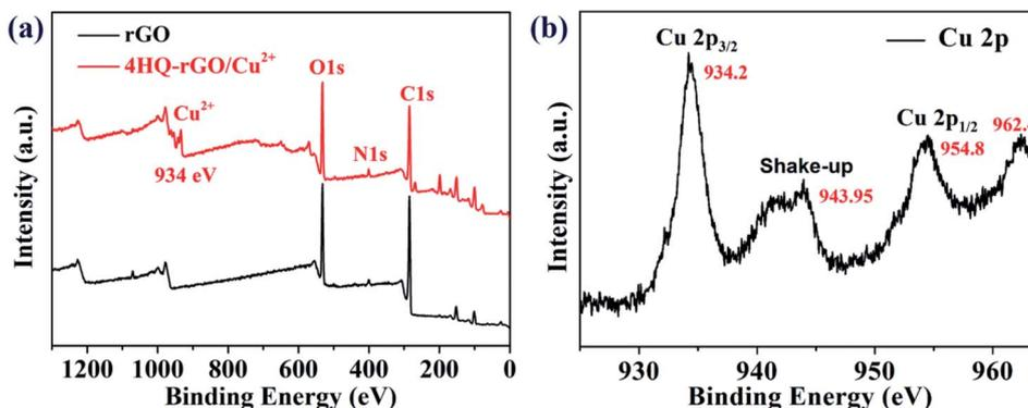
Fig. 4 (a) XPS spectra of the rGO and 4HQ-rGO/Cu<sup>2+</sup> materials. (b) Typical XPS survey scan spectrum of Cu 2p.
