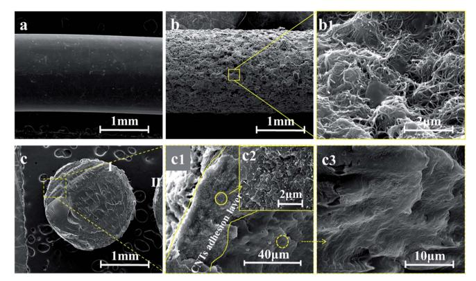
Fig. 2 SEM micrographs of the filament surface before (a) and after (b and b1) CNTs deposition; the corresponding fractured surface of the filament after deposition (c-c3)
