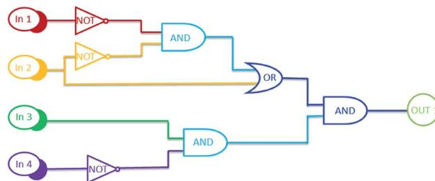
Fig. 6 The logic circuit based on the diarylethene molecule with various inputs: the combinational logic circuits equivalent to the truth table given in Table 2: In 1 (UV), In 2 (Vis), In 3 ( $\text{Al}^{3+}/\text{Zn}^{2+}$ ), In 4 (EDTA), and OUT 1.
