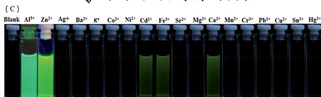
Fig. 2 Changes in the fluorescence of **10** induced by the addition of various metal ions (5.0 equiv.) in ( $2.0 \times 10^{-5} \text{ mol L}^{-1}$ ) methanol: (A) emission spectral changes, (B) emission intensity changes, and (C) photographs of fluorescence changes.
