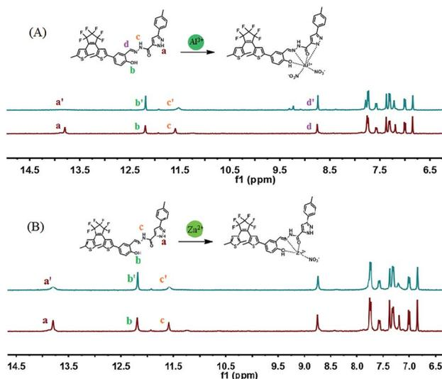
Fig. 5 (A)  $^1\text{H}$  NMR spectra (400 MHz) measured during the titration of **1O** with  $\text{Al}^{3+}$  in  $\text{DMSO}-d_6$ . (B)  $^1\text{H}$  NMR spectra (400 MHz) measured during the titration of **1O** with  $\text{Zn}^{2+}$  in  $\text{DMSO}-d_6$ .
