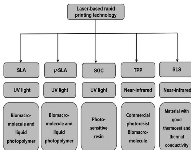
Fig. 1 Classification of laser-based rapid printing technologies.
