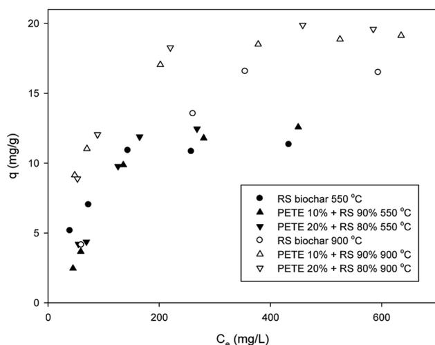
Fig. 2 Removal of DCP by PETE/RS-derived biochar.
