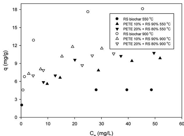
Fig. 1 Removal of DNT by PETE/RS-derived biochar.
