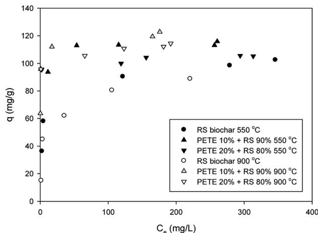
Fig. 4 Removal of Pb by PETE/RS-derived biochar.
