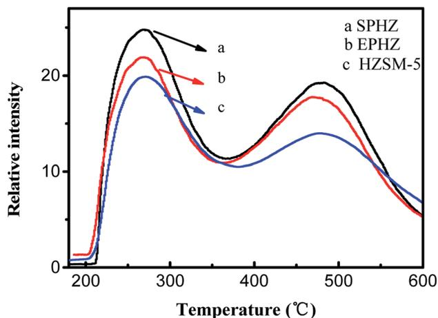
Fig. 6 NH<sub>3</sub>-TPD profiles of HZSM-5, EPHZ and SPHZ.
