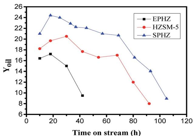
Fig. 9 Time course for the liquid hydrocarbons on HZSM-5, EPHZ and SPHZ. Reaction conditions: 400 °C, 0.1 MPa, WHSV = 1 h<sup>-1</sup>.
