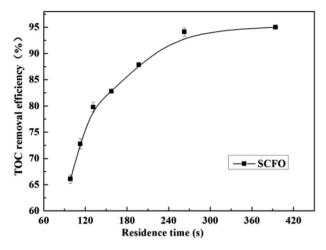
Fig. 4 Effect of residence time on the TOC removal efficiency of the wastewater (420  $^{\circ}$ C, 23.0 MPa, oxidant multiple 4, Fe<sup>2+</sup> 0.30 mg L<sup>-1</sup>, pH 3.0).
