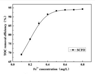
Fig. 5 Effect of  $Fe^{2+}$  concentration on the TOC removal efficiency of wastewater (420 °C, 23.0 MPa, oxidant multiple 4, residence time 197.0 s, pH 3.0).
