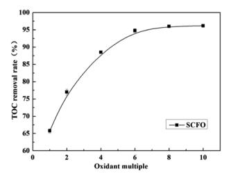
Fig. 3 Effect of oxidant multiple on the TOC removal efficiency of the wastewater (420 °C, 23.0 MPa, flow rate 2.0 mL min<sup>-1</sup>, Fe<sup>2+</sup>  $0.30 \text{ mg L}^{-1}$ , pH 3.0).
