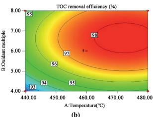
Fig. 9  $\,$  3D (a) and contour plots (b) for TOC removal efficiency as a function of temperature and oxidant multiple interaction (residence time 262.6 s and Fe<sup>2+</sup> 0.5 mg L<sup>-1</sup>).
