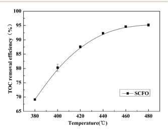
Fig. 2 Effect of temperature on TOC removal efficiency of the wastewater (23.0 MPa, oxidant multiple 4, flow rate 2.0 mL min<sup>-1</sup>, Fe<sup>2+</sup> 0.30 mg L<sup>-1</sup>, pH 3.0).
