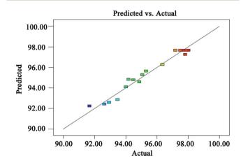
Fig. 8 Predicted value *versus* experimental result of TOC removal efficiency.
