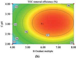
Fig. 11 3D (a) and contour plots (b) for TOC removal efficiency as a function of oxidant multiple and pH interaction (residence time 262.6 s and  $\text{Fe}^{2+}$   $0.5 \text{ mg L}^{-1}$ ).
