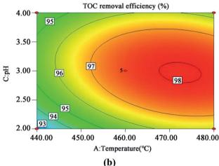
Fig. 10  $\,$  3D (a) and contour plots (b) for TOC removal efficiency as a function of temperature and pH interaction (residence time 262.6 s and Fe<sup>2+</sup> 0.5 mg L<sup>-1</sup>).
