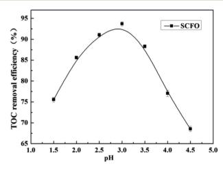
Fig. 6 Effect of pH on the TOC removal efficiency of the wastewater (420  $^{\circ}$ C, 23.0 MPa, oxidant multiple 4, residence time 197.0 s, Fe<sup>2+</sup> 0.30 mg L<sup>-1</sup>).
