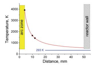
Fig. 9 Temperature distribution in the jet.
