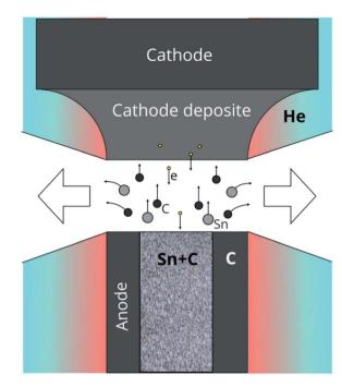
Process of the anode sputtering and fan-shaped jet formation.
