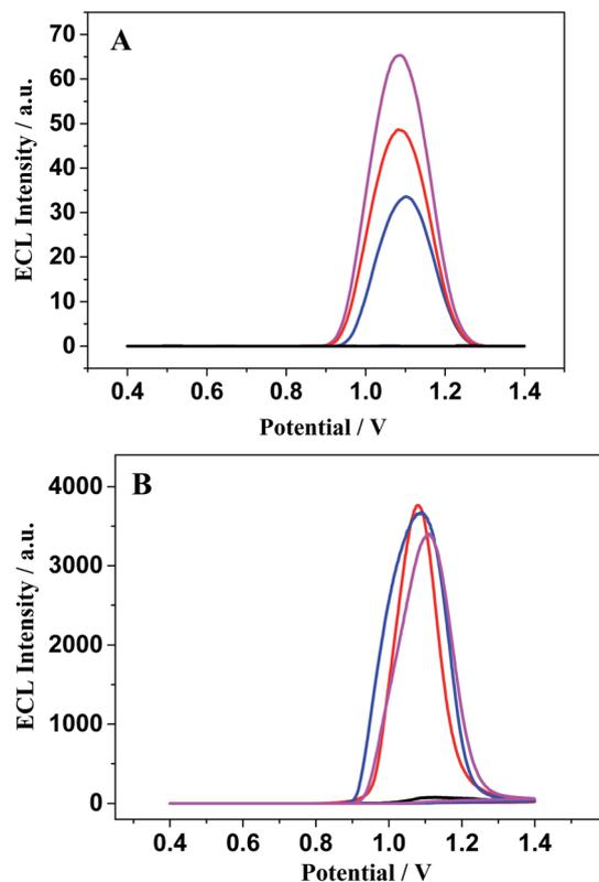
Fig. 8 The ECL signals of different modified electrode: ssDNA/Au (black), WM-DNA/Au (red), MM-DNA/Au (blue) and Abasic-DNA/Au (pink) immersed in  $[\text{Ru}(\text{bpy})_3\text{-GQD}]^{2+}$  (A) and  $[\text{Ru}(\text{bpy})_3]^{2+}$  (B) for 10 min before measurement. The detection was performed in 0.1 M PBS (pH 7.4) containing 0.1 M TPA.
