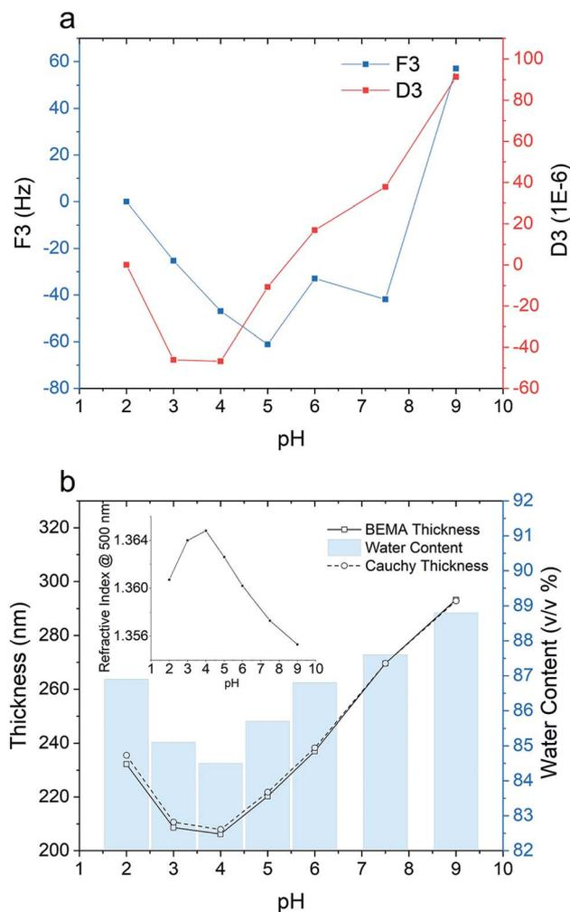
Fig. 7 pH responsiveness of a m-PPEGMEMA/alginate multilayered film; (a) frequency and dissipation changes obtained from QCM-D; (b) Cauchy thickness (circle, dashed line), BEMA thickness (square, solid line) and water content (blue bar). The inset shows how the refractive index changes with the pH variation.
