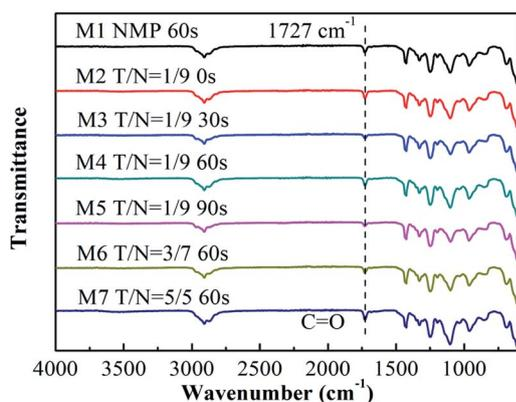
**Fig. 1** FTIR-ATR spectra of the blended membranes at different THF : NMP ratios and different solvent evaporation time. M1, NMP, 60 s; M2, T/N = 1 : 9, 0 s; M3, T/N = 1 : 9, 30 s; M4, T/N = 1 : 9, 60 s; M5, T/N = 1 : 9, 90 s; M6, T/N = 3 : 7, 60 s; M7, T/N = 5 : 5, 60 s.
