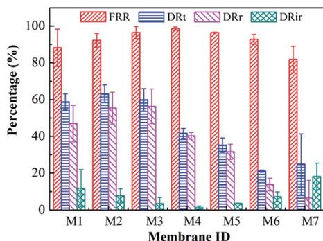
Fig. 7 Characterization of the membrane antifouling properties: the flux recovery ratio (FRR), total flux decline ratio (DR<sub>t</sub>), reversible flux decline ratio (DR<sub>r</sub>), and irreversible flux decline ratio (DR<sub>ir</sub>). M1, NMP, 60 s; M2, T/N = 1 : 9, 0 s; M3, T/N = 1 : 9, 30 s; M4, T/N = 1 : 9, 60 s; M5, T/N = 1 : 9, 90 s; M6, T/N = 3 : 7, 60 s; M7, T/N = 5 : 5, 60 s.
