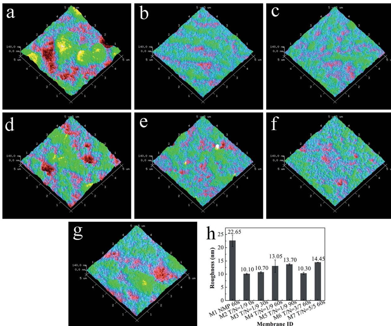
Fig. 4 AFM images of all blended membranes: (a) M1, NMP, 60 s; (b) M2, T/N = 1/9, 0 s; (c) M3, T/N = 1/9, 30 s; (d) M4, T/N = 1/9, 60 s; (e) M5, T/N = 1/9, 90 s; (f) M6, T/N = 3/7, 60 s; (g) M7, T/N = 5/5, 60 s; (h) the RMS roughness of all blended membranes.
