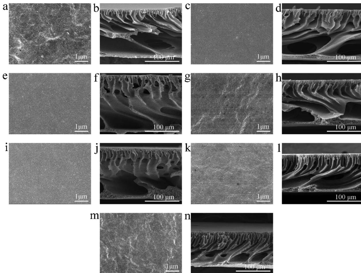
Fig. 3 Surface and cross-sectional morphologies of all blended membranes: (a and b) M1, NMP, 60 s; (c and d) M2, T/N = 1/9, 0 s; (e and f) M3, T/N = 1/9, 30 s; (g and h) M4, T/N = 1/9, 60 s; (i and j) M5, T/N = 1/9, 90 s; (k and l) M6, T/N = 3/7, 60 s; (m and n) M7, T/N = 5/5, 60 s.
