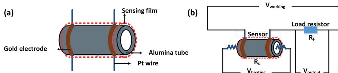
Fig. 1 (a) A schematic diagram of the gas sensor and (b) the electric circuit used to investigate the gas sensor.
