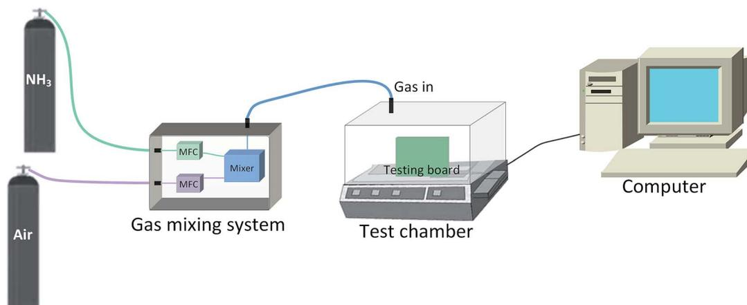
Fig. 2 The experimental setup for gas sensing measurements.
