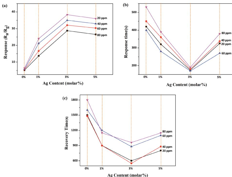
Fig. 5 A performance comparison between Ag-decorated TiO<sub>2</sub> QDs gas sensors with different volumes of Ag addition to NH<sub>3</sub>: (a) response; (b) response time; and (c) recovery time.
