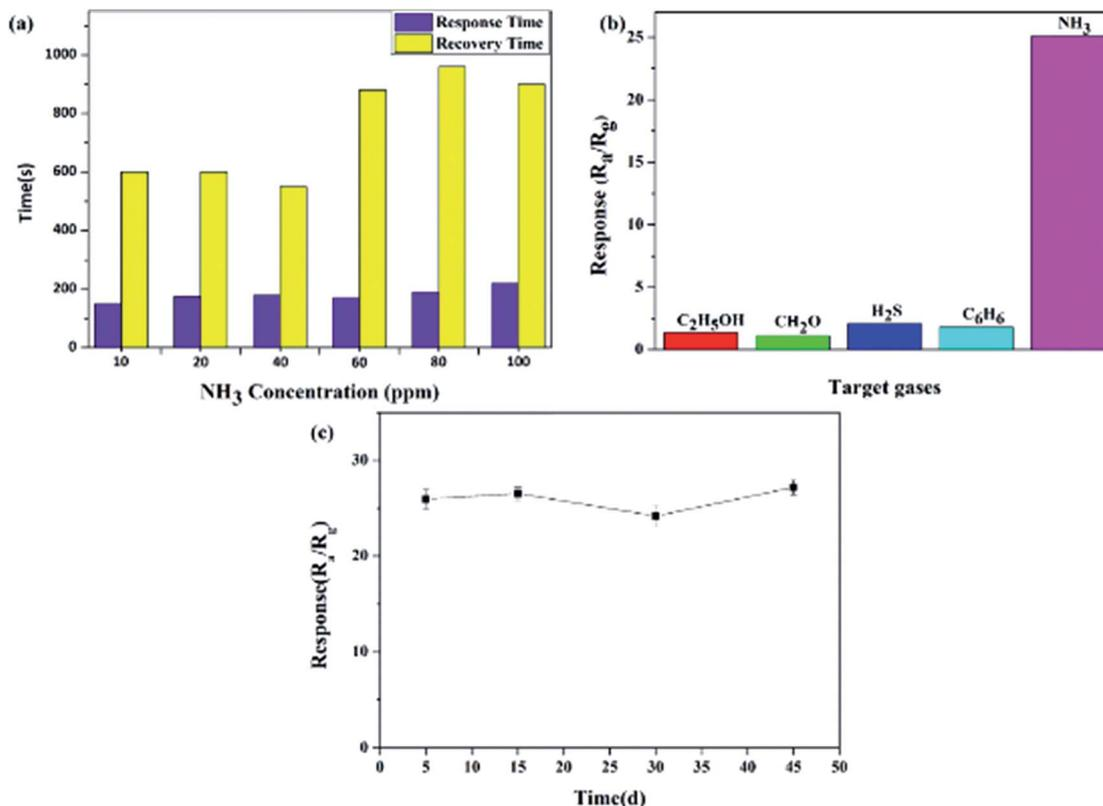
Fig. 7 The gas sensing properties of the Ag-decorated TiO<sub>2</sub> QDs gas sensor: (a) response/recovery time at different NH<sub>3</sub> gas concentrations; (b) selectivity to different gases at 10 ppm; and (c) stability towards 10 ppm NH<sub>3</sub>.
