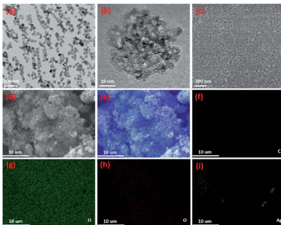
Fig. 4 TEM images of (a)  $\text{TiO}_2$  QDs and (b) a single nanoparticle. An SEM image of (c) Ag-decorated  $\text{TiO}_2$  QDs film. The EDS results from an Ag-decorated  $\text{TiO}_2$  sensing material sample: (d) SEM image; (e) overall mapping; and (f–i) EDS elemental mapping images of C, Ti, O and Ag.
