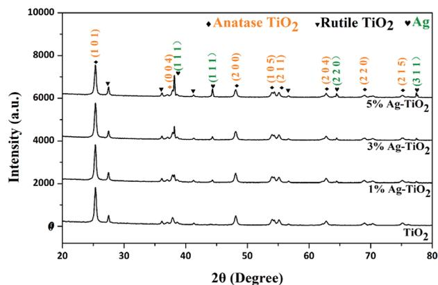
Fig. 3 The XRD patterns of the  $\text{TiO}_2$  QDs and the Ag-decorated  $\text{TiO}_2$  QDs sensing materials.
