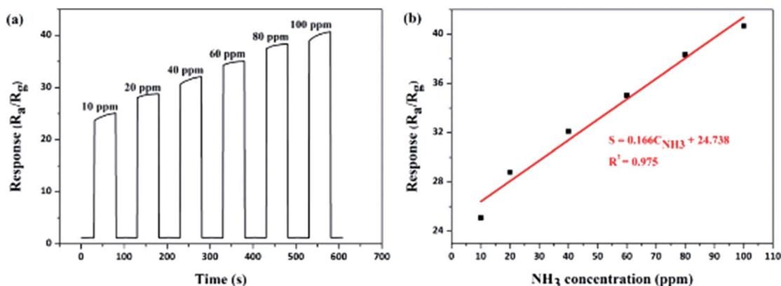
Fig. 6 Gas sensing properties of the Ag-decorated TiO<sub>2</sub> QDs gas sensor to different concentrations of NH<sub>3</sub> gas: (a) dynamic response; and (b) the correlation between the response and concentration.
