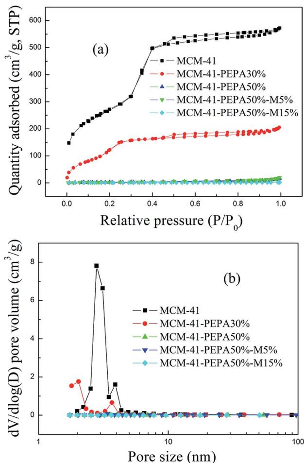
Fig. 1 (a) N<sub>2</sub> adsorption–desorption isotherms and (b) pore size distribution curves for MCM-41 before and after loading.
