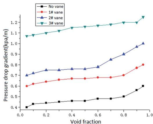
Fig. 10 The relationship between vane and pressure drop.
