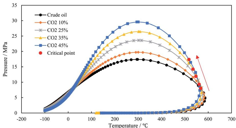
**Fig. 3** Phase behavior of crude oil and CO<sub>2</sub> system at different CO<sub>2</sub> mole fractions.
