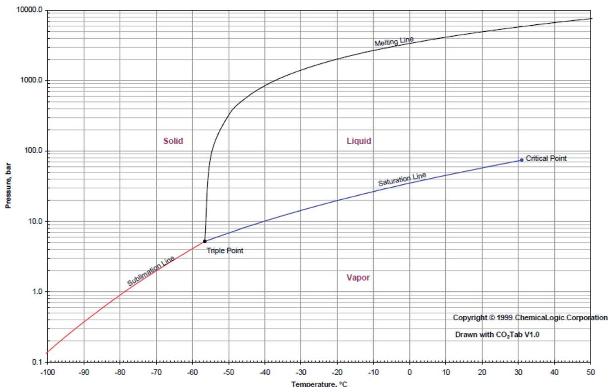
Fig. 1 CO<sub>2</sub> P-T phase behavior diagram (Copyright ©1999 ChemicalLogic Corporation).
