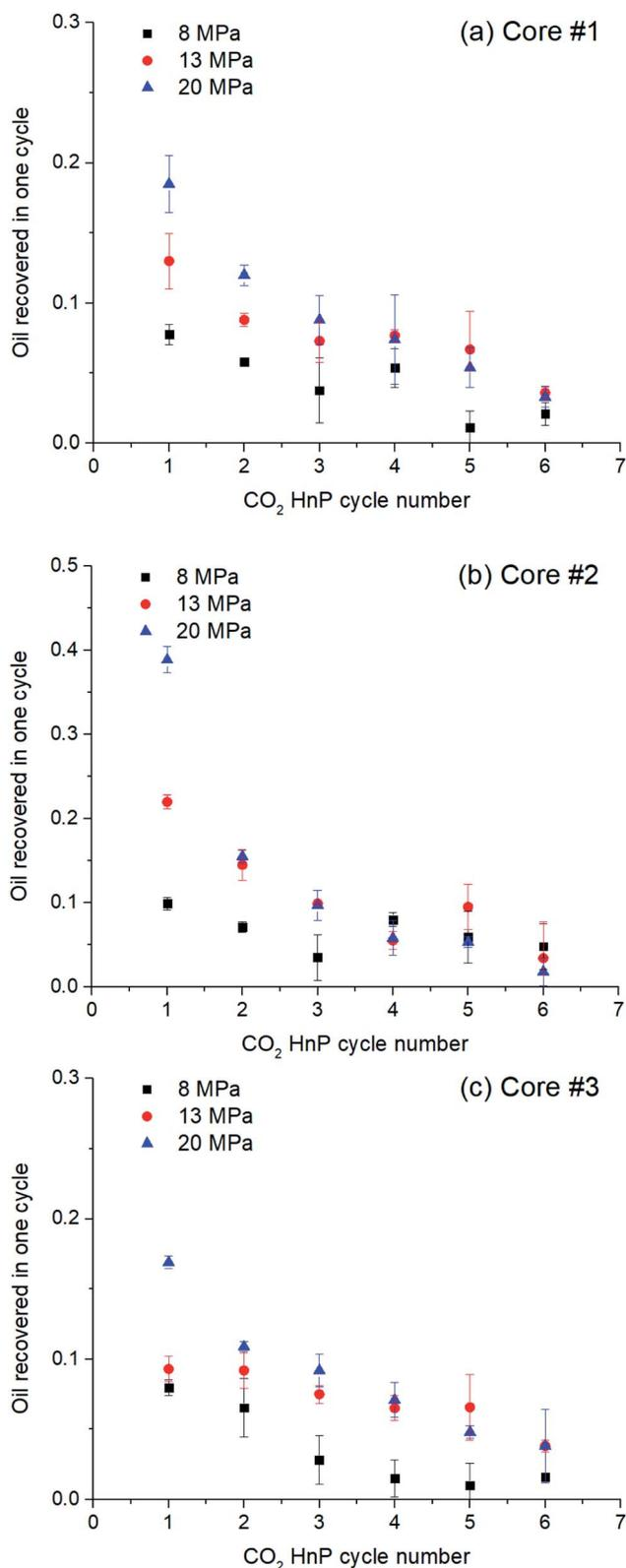
Fig. 11 Oil recovered amount in one cycle during CO<sub>2</sub> HnP at different injection pressures.
