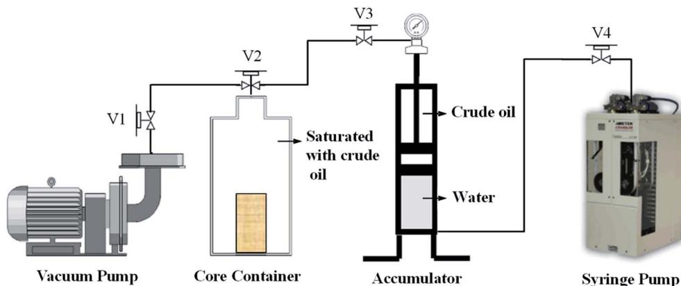
Fig. 8 Schematic diagram of saturated oil experimental equipment.
