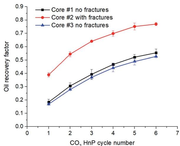
Fig. 14 Matrix permeability and fracture effect on CO<sub>2</sub> huff-n-puff performance at different HnP cycle ( $P = 20 \text{ MPa}$ , soaking time = 0.5 h).
