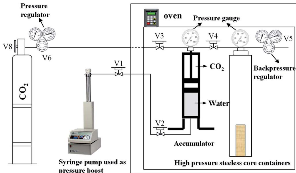
Fig. 9 Schematic of the set up for the CO<sub>2</sub> HnP experiments.
