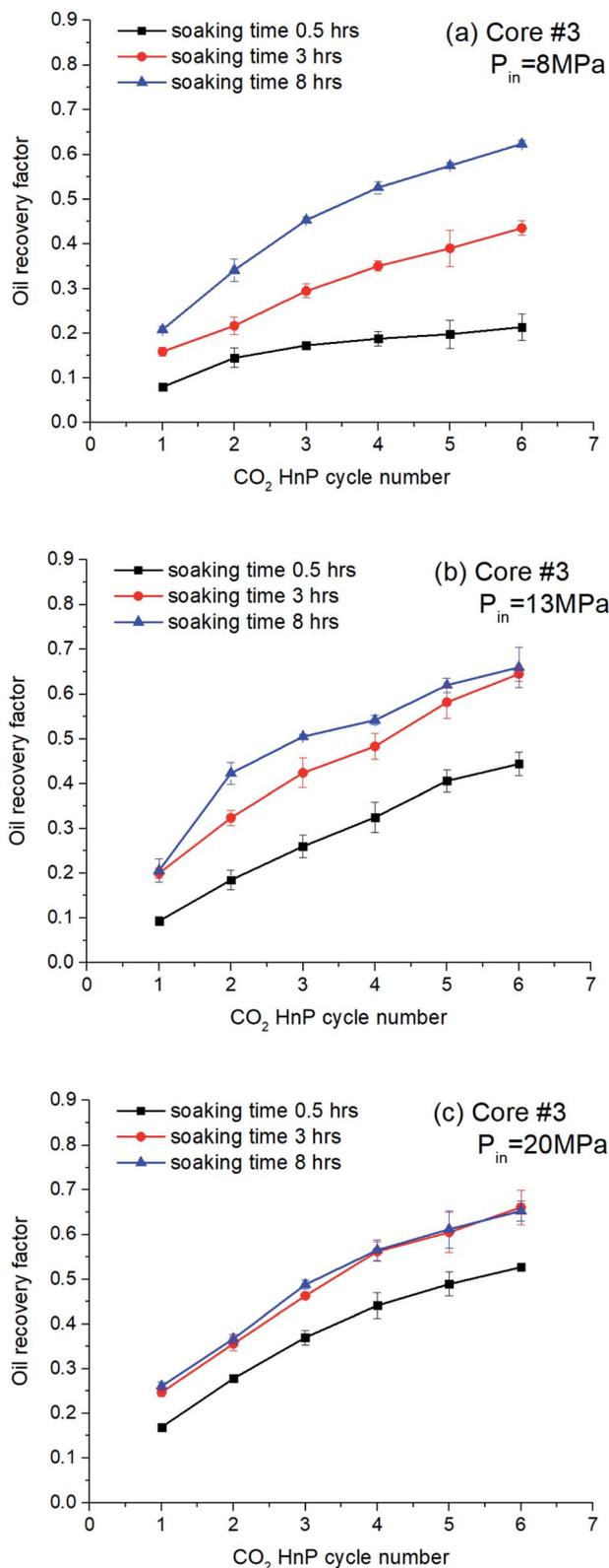
Fig. 12 Soaking time effect on the CO<sub>2</sub> HnP performance with different pressure (Core #3).
