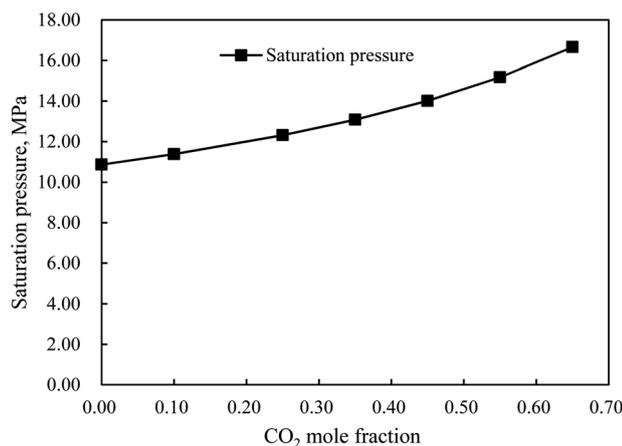
Fig. 6 The changes of formation oil saturation pressure at different CO<sub>2</sub> mole fractions.
