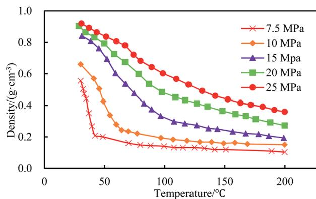
Fig. 2 Density distribution curves under different pressures of CO<sub>2</sub>.
