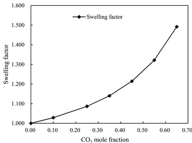
Fig. 5 The changes of formation oil swelling factor at different CO<sub>2</sub> mole fractions.
