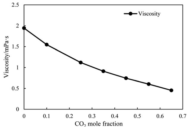
**Fig. 4** The changes of formation oil viscosity with different CO<sub>2</sub> mole fractions at reservoir condition ( $P = 18.62$  MPa,  $T = 69.9$  °C).
