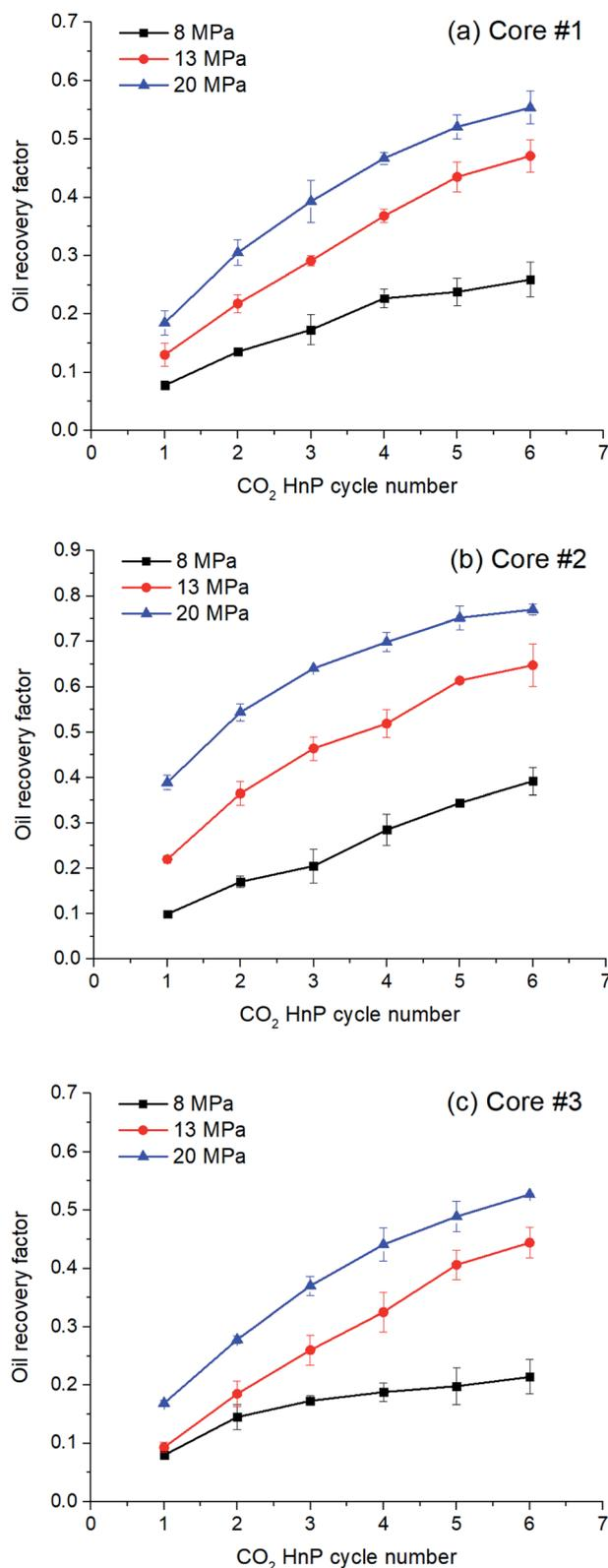
Fig. 10 Oil recovery factor curves of CO<sub>2</sub> HnP at different injection pressures.
