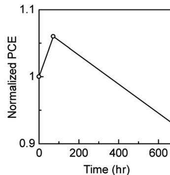
Fig. 4 Normalized power conversion efficiency (PCE) of sealed perovskite solar cells having  $\text{Cs}_{0.05}\text{FA}_{0.79}\text{MA}_{0.16}\text{Pb}(\text{I}_{0.84}\text{Br}_{0.16})_3$  (FA = formamidinium, MA = methylammonium) as light absorber, stored under ambient condition.
