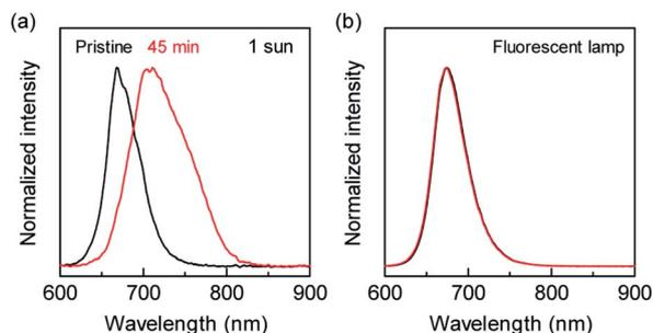
Fig. 3 Photoluminescence (PL) spectra of  $\text{Cs}_{0.05}\text{FA}_{0.79}\text{MA}_{0.16}\text{Pb}(\text{I}_{0.84}\text{Br}_{0.16})_3$  (FA = formamidinium, MA = methylammonium) films exposed to (a) AM 1.5G and (b) fluorescent lamp illumination. The black and red lines represent PL spectra of before and after light soaking, respectively.
