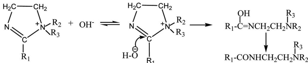
Fig. 5 Hydrolysis reaction of imidazoline quaternary ammonium salt in the presence of water.
