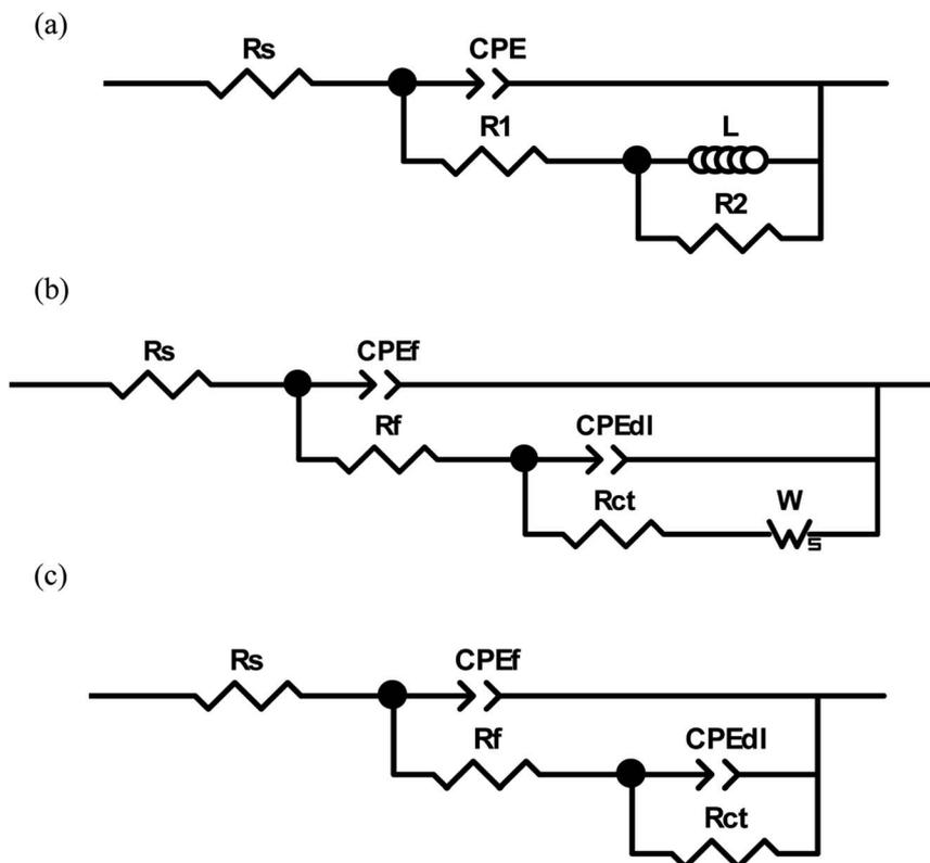
Fig. 9 Equivalent circuits used for modeling of the impedance data.
