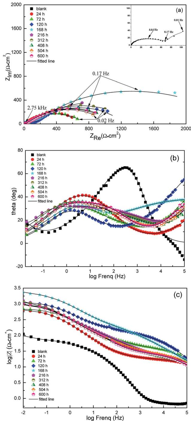
Fig. 8 EIS spectra plots for Q235 steel in  $\text{CO}_2$ -saturated 2% NaCl solution in the presence of  $1000 \text{ mg L}^{-1}$  LFA at different immersion times at 333 K: (a) Nyquist plots (b) Bode phase angle plots, (c) Bode modulus.
