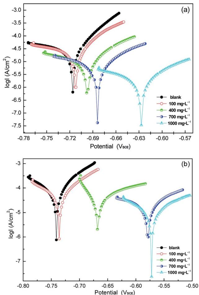
Fig. 6 Weak polarization curves of Q235 steel in CO<sub>2</sub>-saturated solution with varying concentrations of LFA inhibitor at (a) 293 K and (b) 333 K.
