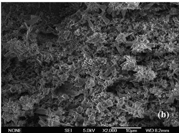
Fig. 10 SEM images for Q235 steel after being corroded in CO<sub>2</sub>-saturated 2% NaCl solution for 72 h at (a) 293 K and (b) 333 K.
