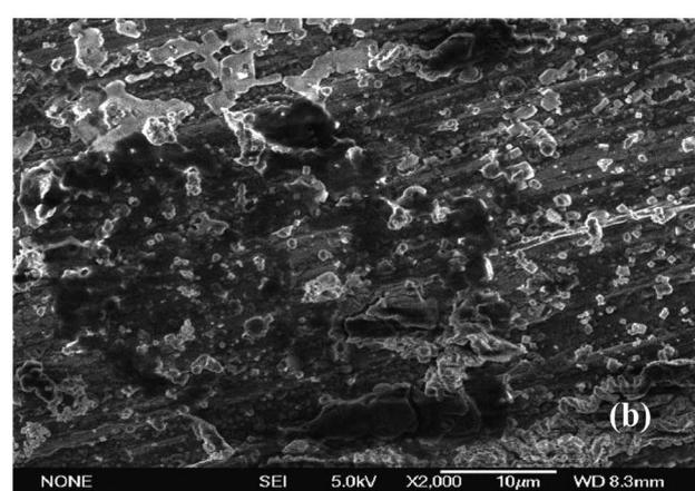
Fig. 11 SEM images for Q235 steel after being corroded in CO<sub>2</sub>-saturated 2% NaCl solution in the presence of 1000 mg L<sup>-1</sup> LFA inhibitor for 72 h at (a) 293 K and (b) 333 K.
