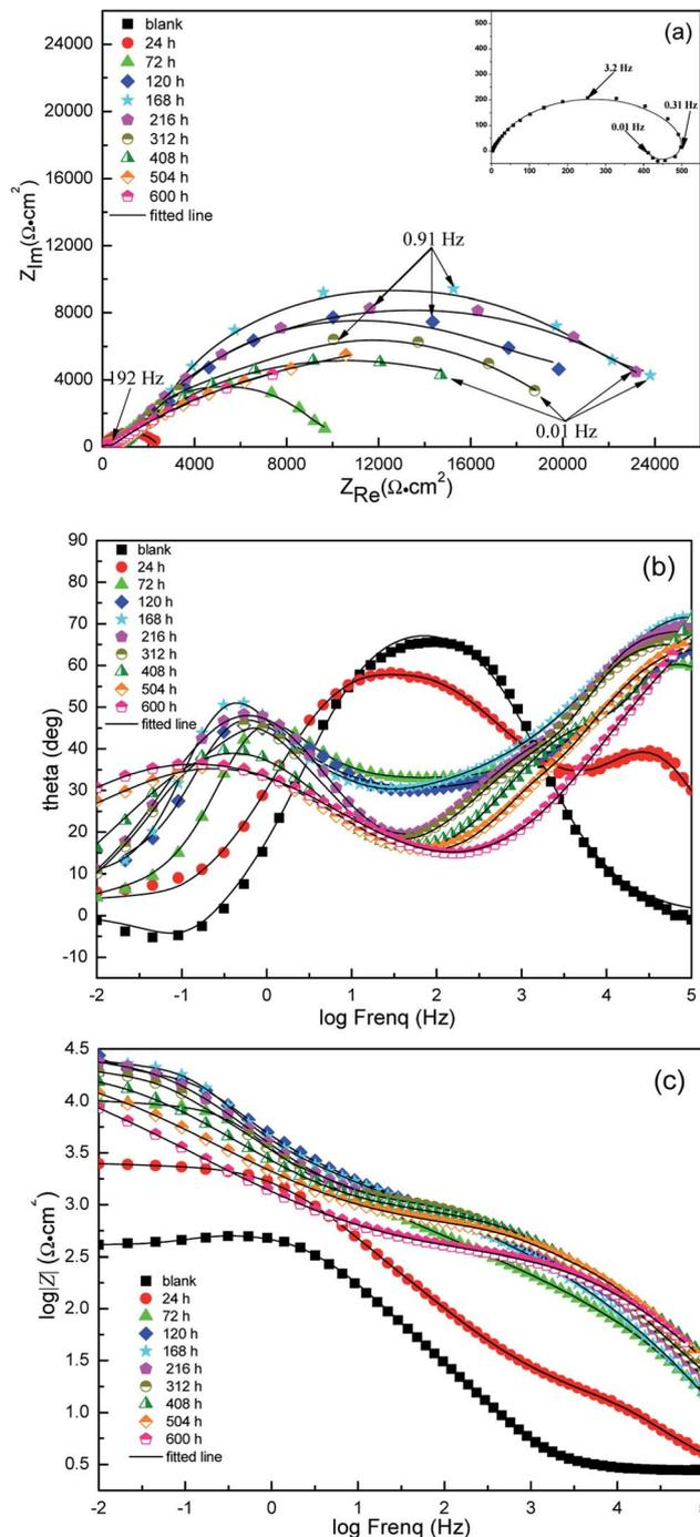
Fig. 7 EIS spectra plots for Q235 steel in  $\text{CO}_2$ -saturated 2% NaCl solution in the presence of  $1000 \text{ mg L}^{-1}$  LFA at different immersion times at 293 K: (a) Nyquist plots (b) Bode phase angle plots, (c) Bode modulus.
