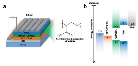
(a) Schematic device structure. (b) Energy diagram of each layer of the LED device. The energy level of CsPbBr<sub>3</sub> are cited from ref. 61.
