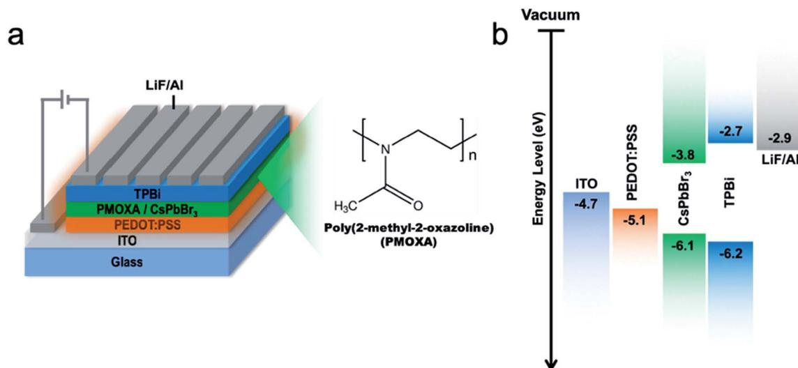
Fig. 5 (a) Schematic device structure. (b) Energy diagram of each layer of the LED device. The energy level of CsPbBr<sub>3</sub> are cited from ref. 61.
