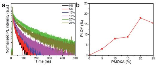
Fig. 2 (a) PL lifetime traced at the emission peak of perovskite films with various concentrations of PMOXA under a fixed excitation fluence of 1  $\mu$ J cm<sup>-2</sup> at the excitation wavelength of 365 nm. (b) PLQYs of CsPbBr<sub>3</sub> films with various concentrations of PMOXA (excited at 1 mW cm<sup>-2</sup>).
