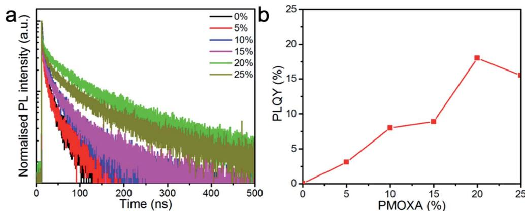
Fig. 2 (a) PL lifetime traced at the emission peak of perovskite films with various concentrations of PMOXA under a fixed excitation fluence of  $1 \mu\text{J cm}^{-2}$  at the excitation wavelength of 365 nm. (b) PLQYs of  $\text{CsPbBr}_3$  films with various concentrations of PMOXA (excited at  $1 \text{ mW cm}^{-2}$ ).
