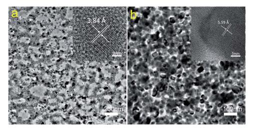
Fig. 4 (a) TEM image of 20% PMOXA-treated CsPbBr<sub>3</sub> film without annealing. Scale bar: 200 nm. Inset image is the high-resolution TEM image of crystal. Scale bar: 3 nm. (b) TEM image of 20% treated-PMOXA CsPbBr<sub>3</sub> film with annealing. Scale bar: 100 nm. Inset image is the high-resolution TEM image of crystal. Scale bar: 5 nm.
