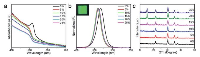
Fig. 1 (a) Absorbances and (b) normalised PL spectra of CsPbBr<sub>3</sub> films with various concentrations of PMOXA. The inserted image is the 20% PMOXA-treated CsPbBr<sub>3</sub> film under UV lamp (365 nm) illumination. (c) XRD patterns of CsPbBr<sub>3</sub> films with various concentrations of PMOXA.
