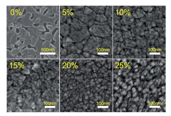
Fig. 3 SEM images of CsPbBr<sub>3</sub> films with various concentrations of PMOXA
