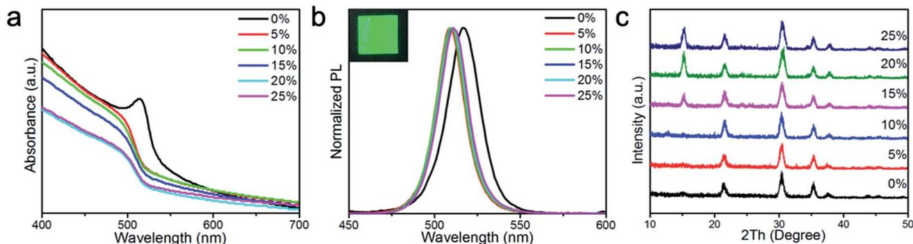
Fig. 1 (a) Absorbances and (b) normalised PL spectra of CsPbBr<sub>3</sub> films with various concentrations of PMOXA. The inserted image is the 20% PMOXA-treated CsPbBr<sub>3</sub> film under UV lamp (365 nm) illumination. (c) XRD patterns of CsPbBr<sub>3</sub> films with various concentrations of PMOXA.
