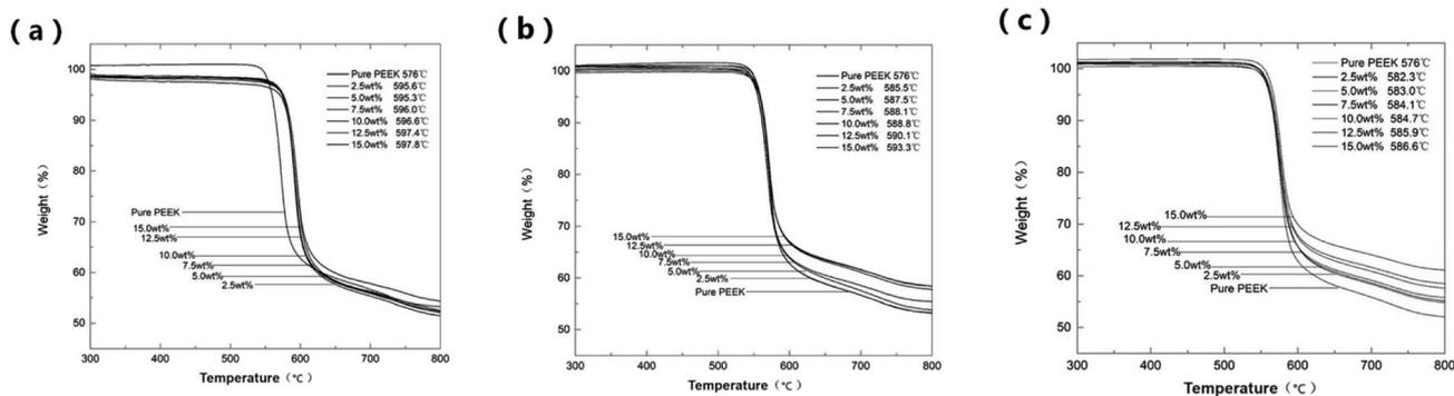
Fig. 1 TGA curves obtained under nitrogen atmosphere of pure PEEK and 3 different types  $\text{Al}_2\text{O}_3$ /PEEK composites: (a) 30 nm  $\text{Al}_2\text{O}_3$  nanoparticle reinforced, (b) 0.2  $\mu\text{m}$   $\text{Al}_2\text{O}_3$  particle reinforced, (c) 5  $\mu\text{m}$   $\text{Al}_2\text{O}_3$  particle reinforced.
