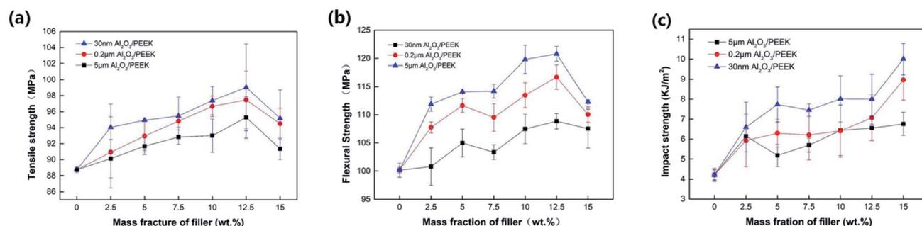
Fig. 4 Tensile strength, flexural strength and impact strength of pure PEEK and  $\text{Al}_2\text{O}_3/\text{PEEK}$  composite with different content: (a) tensile strength, (b) flexural strength, (c) impact strength.
