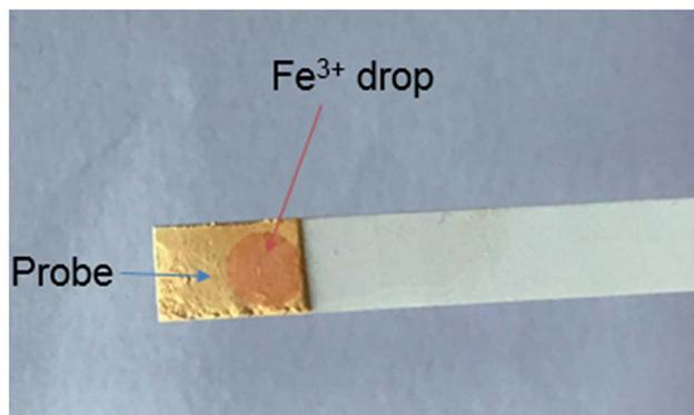
Fig. 6 Photograph of the test strip of this probe **RG5NC** during the detection of Fe<sup>3+</sup>.
