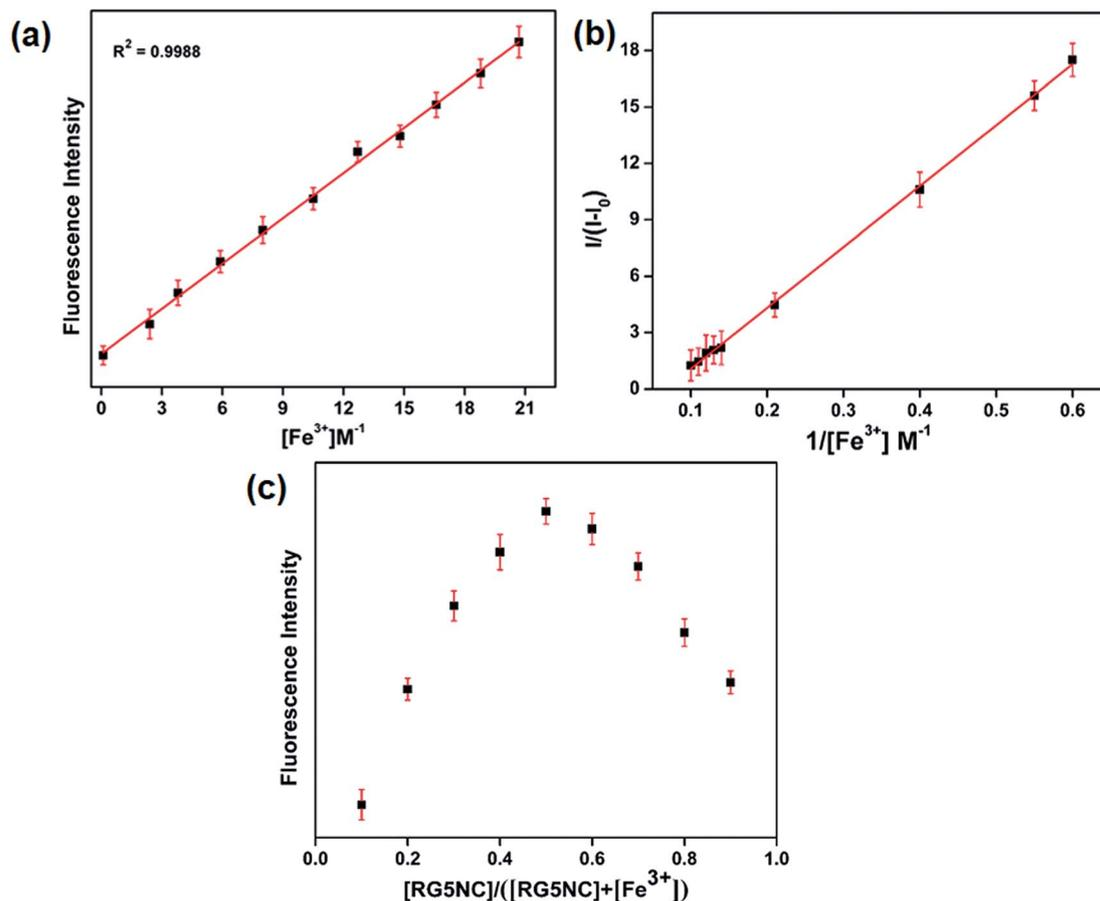
Fig. 2 (a) Fluorescence spectra of RG5NC with various concentration of  $Fe^{3+}$  in MeCN solution varying from 0–20  $\mu M$  (b) Benesi–Hildebrand plot to evaluate binding constant. (c) Job's plot with a total concentration of  $[RG5NC] + [Fe^{3+}] = 20 \mu M$ .
