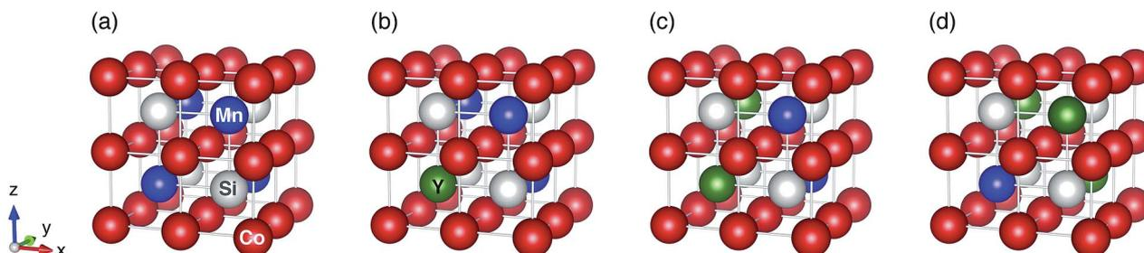
Fig. 1  $L2_1$  symmetric crystal structures for (a) ternary  $\text{Co}_2\text{MnSi}$ , (b) quaternary  $\text{Co}_2(\text{Y}_{0.25},\text{Mn}_{0.75})\text{Si}$ , (c)  $\text{Co}_2(\text{Y}_{0.50},\text{Mn}_{0.50})\text{Si}$ , and (d)  $\text{Co}_2(\text{Y}_{0.75},\text{Mn}_{0.25})\text{Si}$ . Red, blue, white, and green circles indicate Co, Mn, Si, and Y atoms, respectively, where Y is the 3d transition metal atom of Ti, V, Cr, or Fe.
