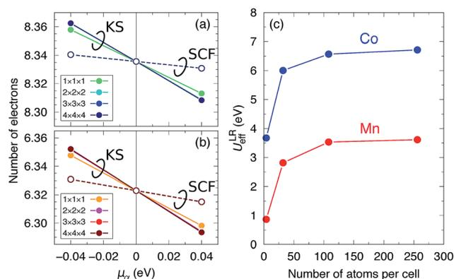
Fig. 2 Variation of the occupied 3d electron numbers on the (a) Co and (b) Mn sites as a function of the applied perturbation potential  $\mu_\alpha$  in  $n \times n \times n$  supercell Co<sub>2</sub>MnSi ( $n = 1, 2, 3, 4$ ). Solid lines indicate the KS calculation terms and dashed ones indicate the SCF terms. (c) The  $U_{\text{eff}}^{\text{LR}}$  value dependence on the number of atoms per cell for Co (blue) and Mn (red).
