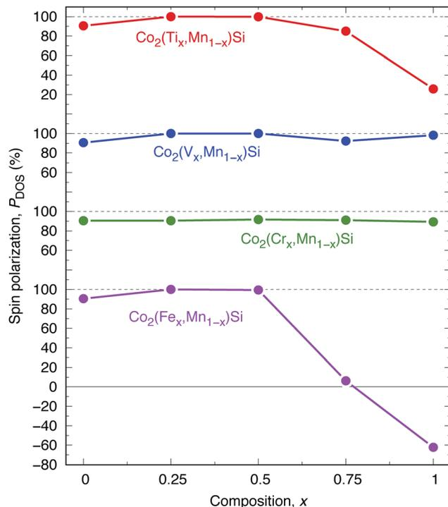
Fig. 11 Spin polarization  $P_{\text{DOS}}$  dependence on composition  $x$  in  $\text{Co}_2(\text{Y}_x\text{Mn}_{1-x})\text{Si}$ . Red, blue, green, and pink plots are  $Y$  of Ti, V, Cr, and Fe, respectively.
