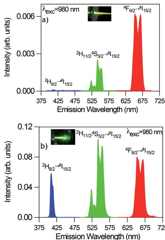
Fig. 7 Room temperature UC emission spectra of GC fibers obtained under excitation at  $980 \text{ nm}$  at two different pump power densities (a)  $2.5 \text{ W cm}^{-2}$  (unfocused) and (b)  $0.75 \text{ kW cm}^{-2}$  (focused).
