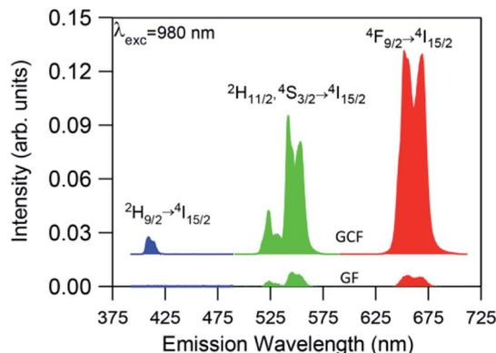
Fig. 5 Room temperature UC emission spectra for the glass (GF) and glass-ceramics fiber (GCF) obtained under excitation at 980 nm with an excitation power density of  $19 \text{ W cm}^{-2}$ . The fibers length was 2 cm.
