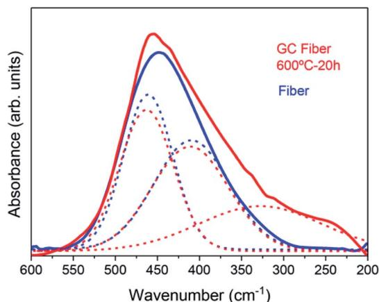
Fig. 3 Comparison of the FTIR spectra of the GC fiber treated at 600 °C for 20 h and of the untreated fiber.
