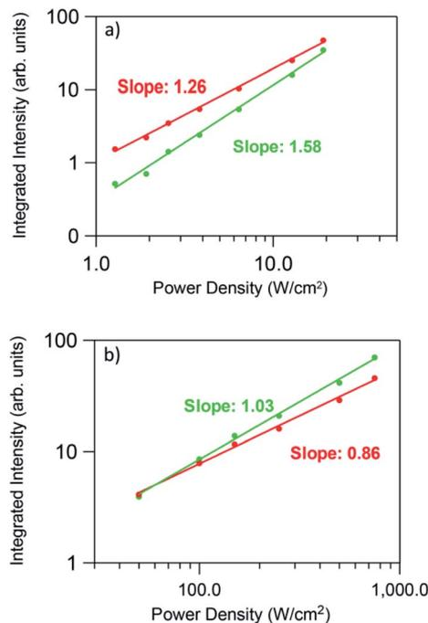
Fig. 10 Dependence of the green and red integrated emission intensities on the excitation power density (a) low pumping regime ( $1.3$  to  $19 \text{ W cm}^{-2}$  unfocused) and (b) high pumping regime ( $0.025$  to  $0.75 \text{ kW cm}^{-2}$  focused).
