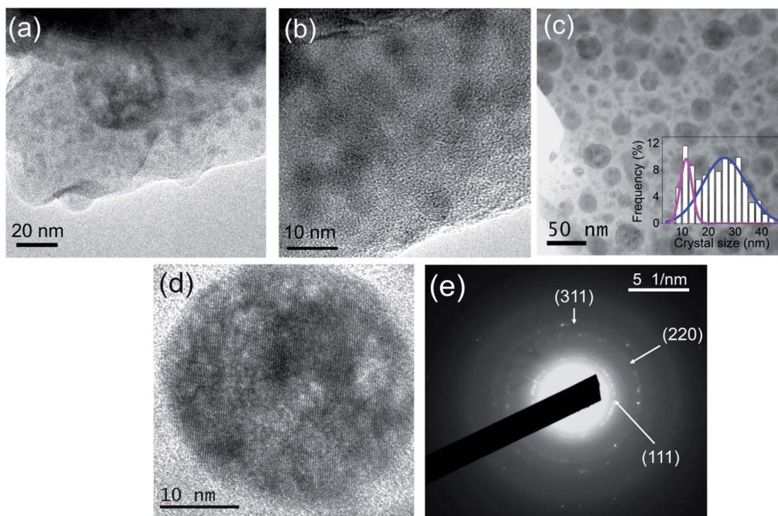
Fig. 4 HRTEM micrograph of the (a and b) as made fiber and (c and d) GC fiber treated at  $600\text{ }^\circ\text{C}$  for 20 h. (e) SAED pattern of GC fiber treated at  $600\text{ }^\circ\text{C}$  for 20 h.
