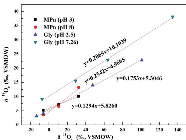
Fig. 2 Plots of  $\delta^{18}\text{O}_\text{P}$  vs.  $\delta^{18}\text{O}_\text{W}$  of phosphates obtained from UVR photo-oxidative hydrolysis of MPn at different pH values and the comparison to the glyphosate data from Sandy' paper.
