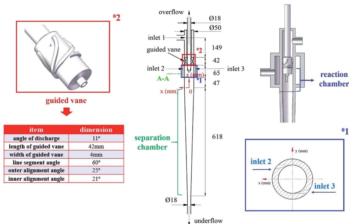
Fig. 1 Schematic diagram of the cyclone reactor structure.
