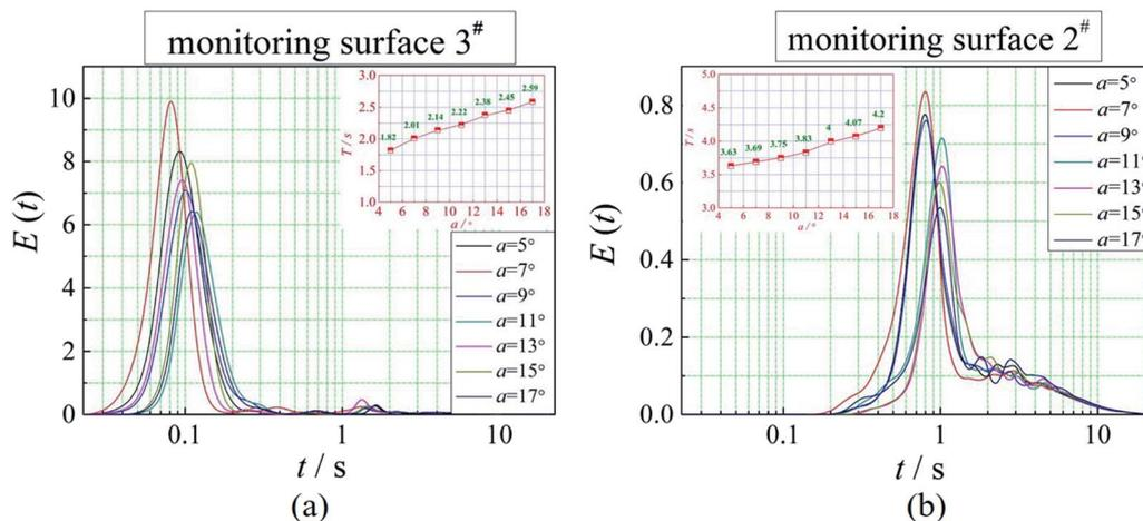
Fig. 8 Effect of  $\alpha$  on the RTD curves.
