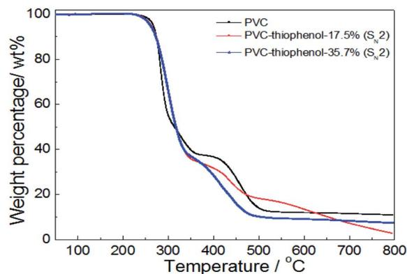
Fig. 5 TG analysis of PVC and the modified PVCs with thiophenol using K<sub>2</sub>CO<sub>3</sub> or DIEA as a base (testing conditions: sample, 10 mg; heating temperature, 50–800 °C; heating rate, 10 °C min<sup>-1</sup>; 50 mL min<sup>-1</sup> N<sub>2</sub> flow).
