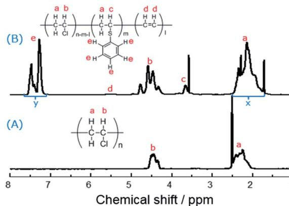
Fig. 2 <sup>1</sup>H NMR spectra of PVC and the modified PVC using thiophenol as a nucleophile (400 MHz, THF-*d*<sub>8</sub>, 329.9 K. Reaction conditions: 500 mg PVC, 1.0 eq. thiophenol, 0.1 eq. K<sub>2</sub>CO<sub>3</sub>, 40 °C, 50 mL DMF as solvent, 3 h).
