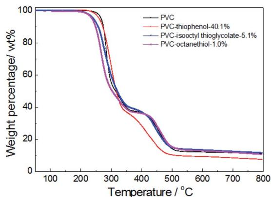
Fig. 4 TG analysis of PVC and the modified PVCs with different nucleophiles using DIEA as a base (testing conditions: sample, 10 mg; heating temperature, 50–800 °C; heating rate, 10 °C min<sup>-1</sup>; 50 mL min<sup>-1</sup> N<sub>2</sub> flow).
