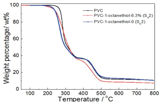
Fig. 6 TG analysis of PVC and the modified PVCs with 1-octanethiol using  $K_2CO_3$  or DIEA as a base (testing conditions: sample, 10 mg; heating temperature, 50–800 °C; heating rate, 10 °C  $min^{-1}$ ; 50 mL  $min^{-1}$   $N_2$  flow).
