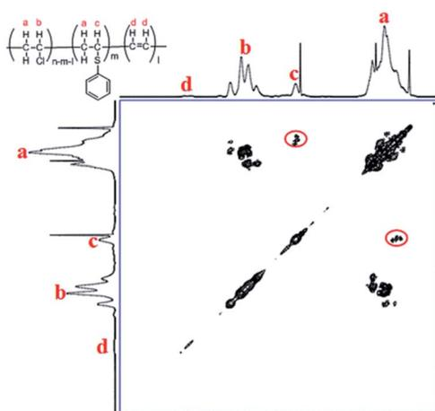
Fig. 3  $^1\text{H}$ - $^1\text{H}$  COSY of PVC and the modified PVC with thiophenol (400 MHz,  $\text{THF-d}_8$ , 353.0 K. Reaction conditions: 500 mg PVC, 1.0 eq. thiophenol, 0.1 eq.  $\text{K}_2\text{CO}_3$ , 40 °C, 50 mL DMF as solvent, 3 h).
