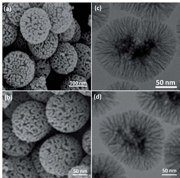
**Fig. 1** FESEM images of  $\text{FeNi}_3/\text{DFNS}$  MNPs (a) and  $\text{FeNi}_3/\text{DFNS}/[\text{Ru}(\text{Bpy})_3]^{2+}$  MNPs (b); TEM images of  $\text{FeNi}_3/\text{DFNS}$  MNPs (c) and  $\text{FeNi}_3/\text{DFNS}/[\text{Ru}(\text{Bpy})_3]^{2+}$  MNPs (d).
