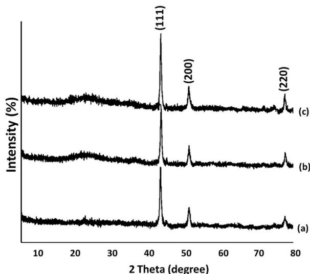
Fig. 3 XRD analysis of (a) FeNi<sub>3</sub>, (b) FeNi<sub>3</sub>/DFNS, and (c) FeNi<sub>3</sub>/DFNS/[Ru(Bpy)<sub>3</sub>]<sup>2+</sup> MNPs.
