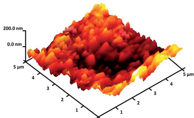
Fig. 4 Three-dimensional AFM image of FeNi<sub>3</sub>/DFNS/[Ru(Bpy)<sub>3</sub>]<sup>2+</sup> MNPs.
