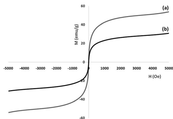
Fig. 6 Room-temperature magnetization curves of (a) FeNi<sub>3</sub> and (b) FeNi<sub>3</sub>/DFNS/[Ru(Bpy)<sub>3</sub>]<sup>2+</sup> MNPs.
