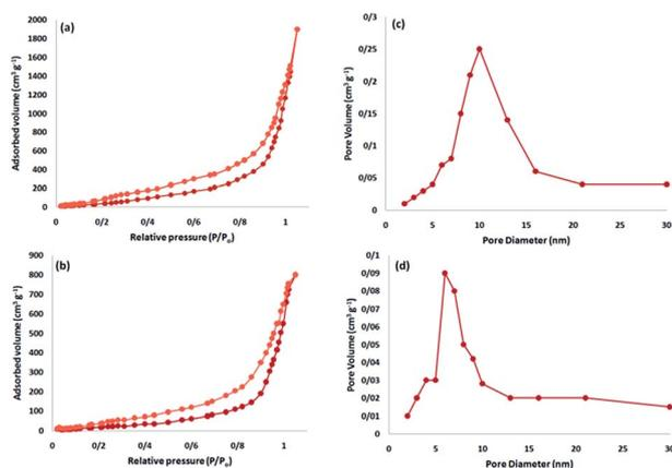
Fig. 8 Adsorption-desorption isotherms of the FeNi<sub>3</sub>/DFNS NPs (a), and FeNi<sub>3</sub>/DFNS/[Ru(Bpy)<sub>3</sub>]<sup>2+</sup> (b); and BJH pore size distributions of the FeNi<sub>3</sub>/DFNS NPs (c), and FeNi<sub>3</sub>/DFNS/[Ru(Bpy)<sub>3</sub>]<sup>2+</sup> MNPs (d).
