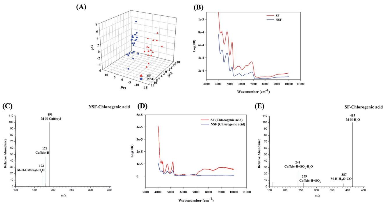
Fig. 4 The MOCA for the FLJ. (A) The discriminatory information of preprocess method of SG9+1<sup>st</sup>; (B) the synchronous 2D-COS auto-peak analysis of the SF and NSF samples; (C) the mass fragmentation behaviors of SF chlorogenic acid; (D) the synchronous 2D-COS auto-peak analysis of the SF and NSF chlorogenic acid samples; (E) the mass fragmentation behaviors of SF chlorogenic acid.
