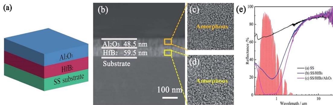
Fig. 1 (a) Schematic diagram of the SS/HfB<sub>2</sub>/Al<sub>2</sub>O<sub>3</sub> absorber coating. (b) Cross-section image of the HfB<sub>2</sub>/Al<sub>2</sub>O<sub>3</sub> absorber coating. HR-TEM images of (c) the HfB<sub>2</sub> layer and (d) Al<sub>2</sub>O<sub>3</sub> layer. (e) The reflectance spectra of the SS, SS/HfB<sub>2</sub> and SS/HfB<sub>2</sub>/Al<sub>2</sub>O<sub>3</sub> coatings.
