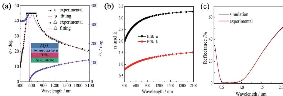
Fig. 3 (a) Experimental and theoretical ellipsometric  $\psi$  and  $\Delta$  spectra for the HfB<sub>2</sub>/Al<sub>2</sub>O<sub>3</sub> layer deposited on Si substrates. (b) The  $n$  and  $k$  values for the HfB<sub>2</sub> layer and (c) experimental and simulated reflectance spectra of the HfB<sub>2</sub>/Al<sub>2</sub>O<sub>3</sub> coating deposited on SS substrates.
