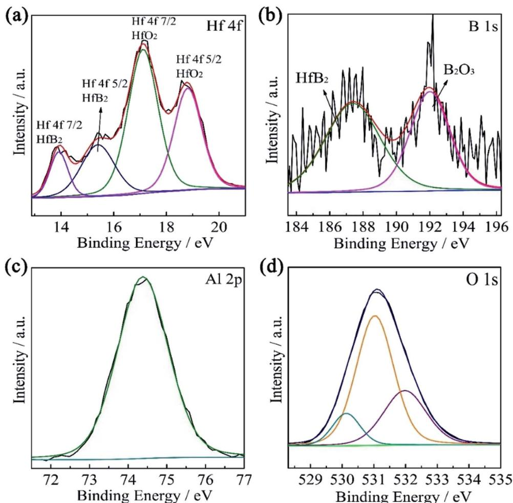
Fig. 2 High-resolution XPS spectra of (a) Hf 4f and (b) B 1s for the single HfB<sub>2</sub> layer and (c) Al 2p and (d) O 1s for the top Al<sub>2</sub>O<sub>3</sub> layer.
