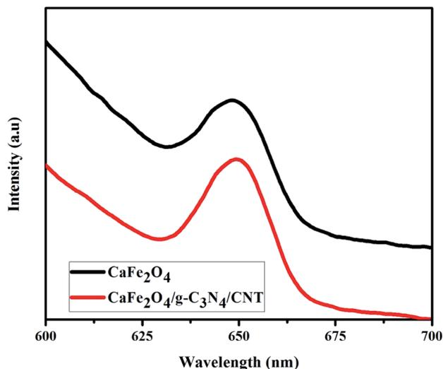
Fig. 8 PL analysis of  $\text{CaFe}_2\text{O}_4$  and  $\text{CaFe}_2\text{O}_4/\text{g-C}_3\text{N}_4/\text{CNTs}$  composite.
