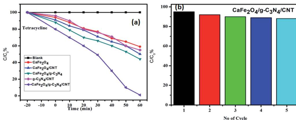
Fig. 13 (a) Adsorption and visible light photocatalytic performance of the samples in the degradation of TC and (b) stability test of the  $\text{CaFe}_2\text{O}_4/\text{g-C}_3\text{N}_4/\text{CNT}$  composite in recycling degradation of TC.
