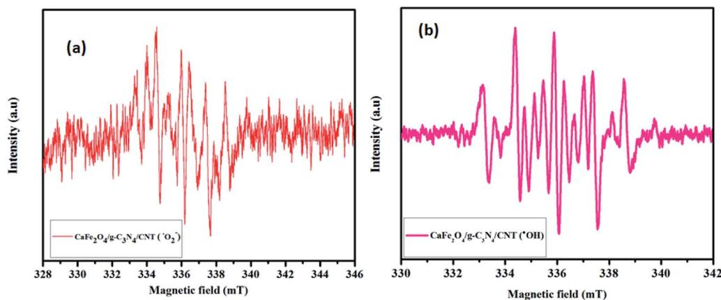
Fig. 11 EPR spectrum of  $\text{CaFe}_2\text{O}_4/\text{g-C}_3\text{N}_4/\text{CNT}$  composite using DMPO.
