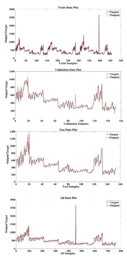
Fig. 2 Target and output nanofiber diameter values for training, validation, and testing sets and all data.
