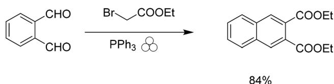
Scheme 2 Mechanochemical synthesis of naphthalene-2,3-dicarboxylic acid diethyl ester.
