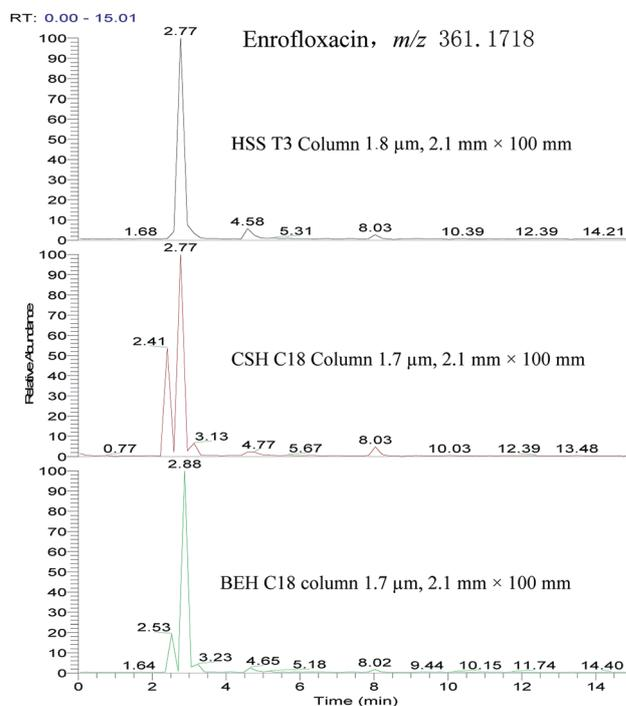
Fig. 2 Extracted ion chromatogram of enrofloxacin performed in different columns in spiked sample ( $10\text{ }\mu\text{g kg}^{-1}$ ).
