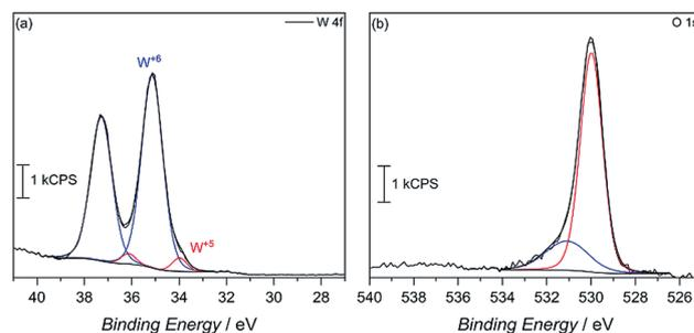
Fig. 4 (a) W 4f and (b) O 1s XPS spectra for the as-synthesized MW-WO<sub>3</sub> particles.
