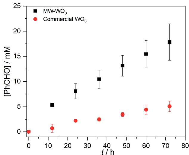
Fig. 5 Benzaldehyde production during the photocatalytic oxidation of benzyl alcohol on MW-WO<sub>3</sub> (black squares) and bulk WO<sub>3</sub> (red circles) using 460 nm blue LEDs.
