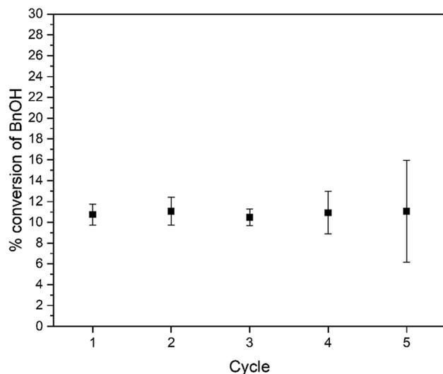
Fig. 6 Recyclability of WO<sub>3</sub> for photocatalytic oxidation of benzyl alcohol.
