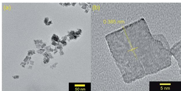
Fig. 8 (a) TEM images of MW- $\text{WO}_3$  particles after photocatalysis on benzyl alcohol. (b) High resolution TEM image of a  $\text{WO}_3$  nanoplatelet after photocatalysis.
