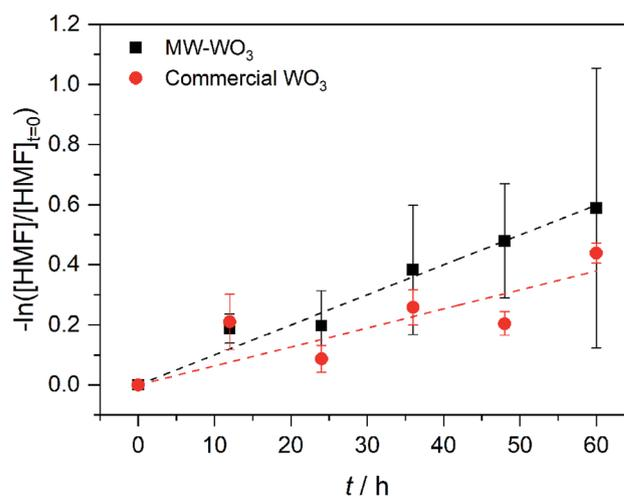
Fig. 7 First order rate plot for the photocatalytic oxidation of HMF on MW-WO<sub>3</sub> (black squares) and bulk WO<sub>3</sub> (red circles) using 460 nm blue LEDs.
