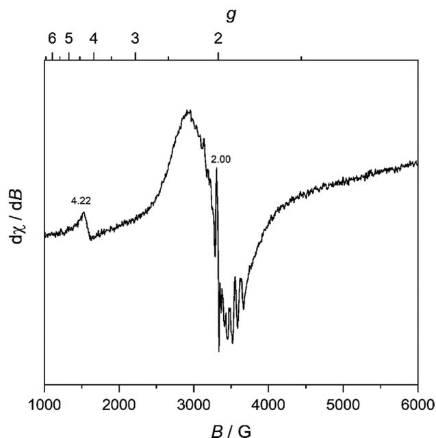
Fig. 3 Room temperature EPR spectra for the as-synthesized MW-WO<sub>3</sub> particles.
