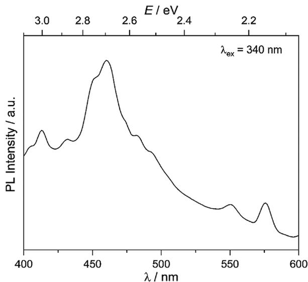
Fig. 2 Room temperature photoluminescence spectra for the as-synthesized MW-WO<sub>3</sub> particles. Spectra were collected with an excitation wavelength of 340 nm.
