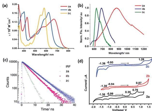
**Fig. 3** (a) UV-Vis absorption spectra (5  $\mu\text{M}$ ) of the PMI derivatives in  $\text{CHCl}_3$  (b) normalized emission spectra (5  $\mu\text{M}$ ) in  $\text{CHCl}_3$  (c) fluorescence lifetime decay plot for the PMI derivatives in toluene and (d) cyclic voltammograms of the compounds in DCM (electrolyte: 0.1 M  $n\text{-Bu}_4\text{NPF}_6$ , ferrocene as the internal), arrows show the direction of CV scan.
