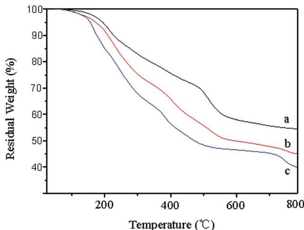
Fig. 9 TG curve of PF (a), 40% NLPF (b), and 40% LPF (c) resins.
