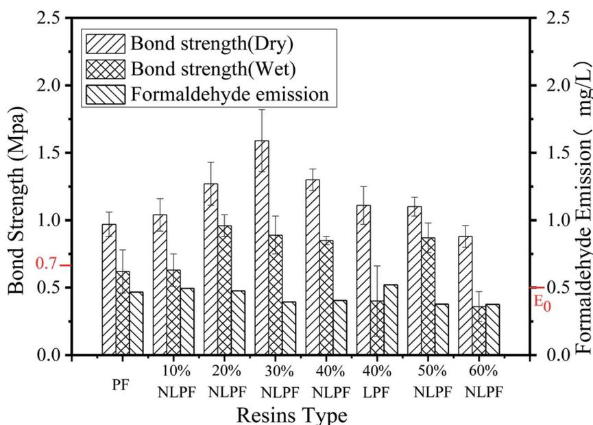
Fig. 7 Bond strength and formaldehyde emission from plywood bonded with PF, LPF, and NLPF resins.
