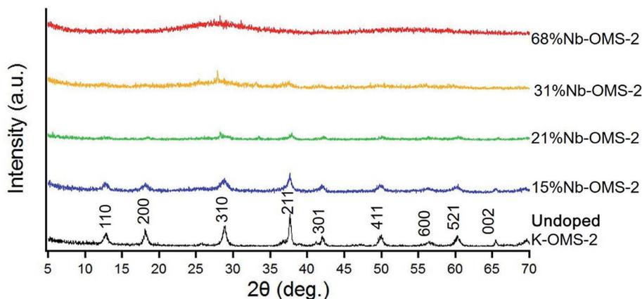
Fig. 1 Powder XRD stack plot of Nb-OMS-2.
