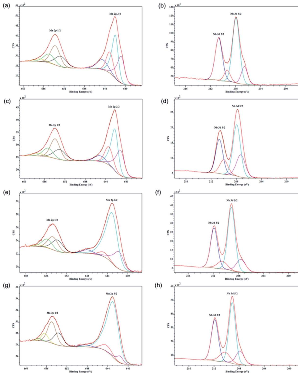
Fig. 4 XPS Spectra of Nb-OMS-2 materials: (a and b) 15% Nb-OMS-2, (c and d) 21% Nb-OMS-2, (e and f) 31% Nb-OMS-2, (g and h) 68% Nb-OMS-2.
