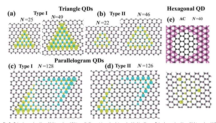
Fig. 2 Spin charge densities of (a) type-I, and (b) type-II silicene triangular dots embedded in silicane. Spin charge densities of (c) type-I and (d) type-II silicene parallelogram QDs embedded in silicane. (e) Spin charge density of hexagonal QD with armchair edges and forty bare Si atoms. The yellow isosurface denote the majority spin, and the blue one is the minority spin.
