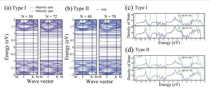
Fig. 5 Band structures of (a) type-I and (b) type-II silicene parallelogram dots embedded in silicane. DOS of parallelogram embedded SiQDs are in (c) for type-I and in (d) for type-II. The green lines in (c) and (d) are the DOS of silicane. The solid magenta lines and dashed blue lines are referred to the majority and minority spin, respectively, for both band dispersion and DOS of QDs. The solid blue lines are for the nomagnetic states.
