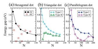
Fig. 7 The  $E_a$  of the (a) hexagonal, (b) triangular, and (c) parallelogram silicene dot embedded in silicane
