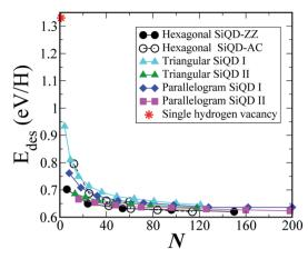
Fig. 8 Desorption energy per hydrogen atom of the SiQD for different shapes of silicene quantum dot embedded in silicane.
