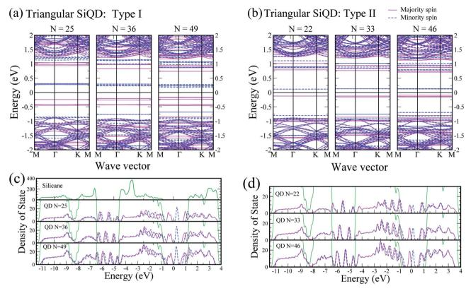
Fig. 4 Band structures of (a) type-I and (b) type-II silicene triangular dots embedded in silicane. Density of states (DOS) of (c) type-I and (d) type-II embedded SiQDs. The DOS of silicane is also shown in (c), and the green lines in (c) and (d) are the DOS of silicane. The magenta solid lines and the blue dash lines refer to the majority and the minority spin states, respectively.
