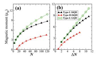
Fig. 3 Total magnetic moment of an embedded SiQD as a function of (a) number of bare Si atoms N, and of (b) the difference of the number of bare Si atoms at A site and at B site ( $\Delta N$ ). The total magnetic moment of type-I embedded graphene triangular QDs is drawn for comparison (green circles).
