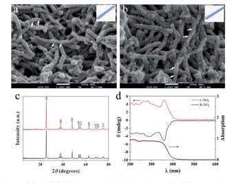
Fig. 1 (a) and (b) SEM images of the helical L- and R-TiO<sub>2</sub> nanofibers and corresponding schematic diagrams of the double-helical structures (insert). X-ray diffraction patterns (c), DRUV-Vis and DRCD spectra (d) of the L- and R-TiO2 nanofibers.
