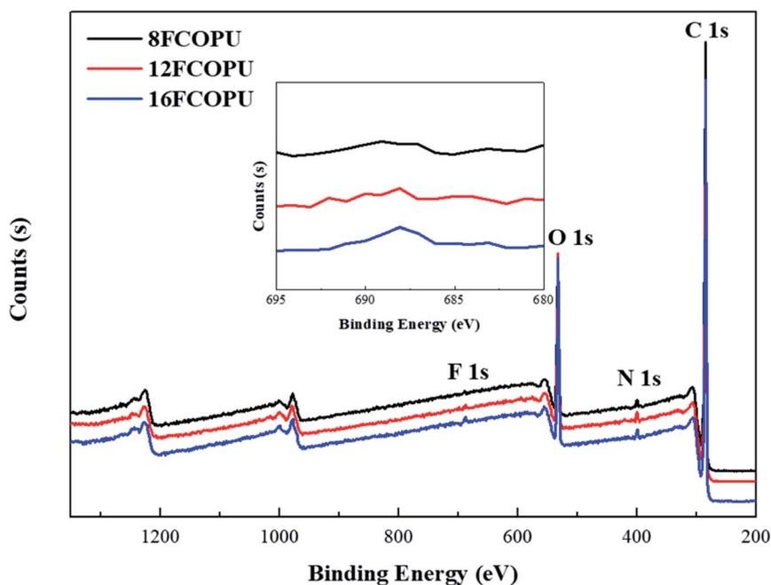
Fig. 7 XPS survey spectra of the FCOPUs.
