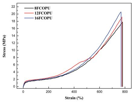
Fig. 13 Tensile properties of the FCOPUs.
