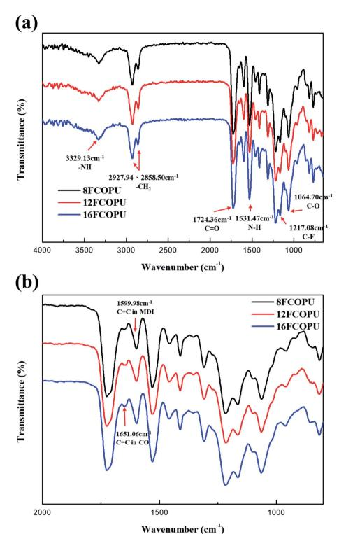
Fig. 5 FT-IR spectra of the FCOPUs at the wavenumber range of (a)  $4000-650 \text{ cm}^{-1}$ ; (b)  $2000-800 \text{ cm}^{-1}$ .
