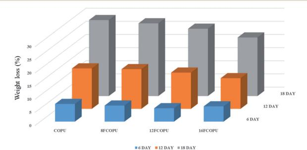
Fig. 14 Weight loss of hydrolytic degradation results of the FCOPUs.
