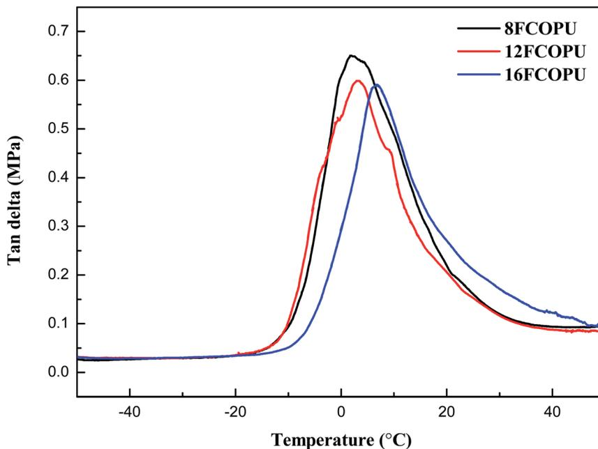
Fig. 12 DMA  $\tan \delta$  curves of the FCOPUs.
