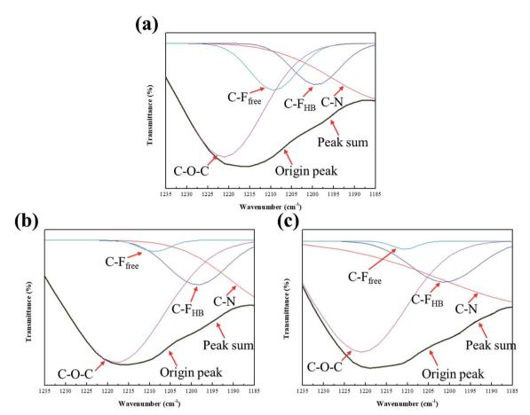
Fig. 6 FT-IR spectra of (a) 8FCOPU; (b) 12FCOPU; (c) 16FCOPU at the wavenumber range of 1235–1185 cm<sup>-1</sup>.
