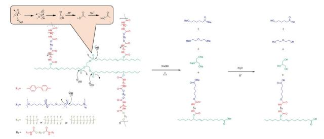
Fig. 15 Degradation mechanism of FCOPUs.
