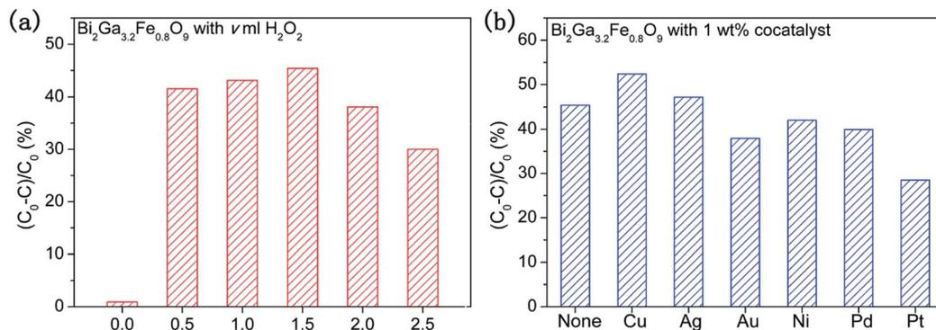
Fig. 5 The conversion efficiency of RhB over the  $\text{Bi}_2\text{Ga}_{3.2}\text{Fe}_{0.8}\text{O}_9$  sample under visible light irradiation: (a) addition of different volumes of  $\text{H}_2\text{O}_2$  in 250 mL solution; (b) loading 1 wt% of different cocatalysts on the photocatalyst. Photocatalytic conditions: 100 mg photocatalyst, 250 mL solution, RhB 20 ppm, pH = 6, 300 W long-arc xenon lamp.
