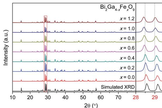
Fig. 1 The powder XRD patterns for the solid solutions, where the simulated XRD pattern for the un-doped  $\text{Bi}_2\text{Ga}_4\text{O}_9$  is also given at the bottom. Also, the inserted red rectangle was magnified to the right of the XRD patterns.
