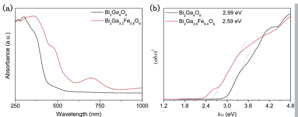
Fig. 3 (a) UV-Vis diffused reflectance spectrum for  $\text{Bi}_2\text{Ga}_4\text{O}_9$  and  $\text{Bi}_2\text{Ga}_{3.2}\text{Fe}_{0.8}\text{O}_9$ . (b) The estimated bandgap energy  $E_g$  with a plot of  $(\alpha h\nu)^2$  against the photon energy ( $h\nu$ ).
