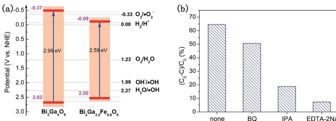
Fig. 7 (a) Schematic illustration of the band structure diagram of Bi<sub>2</sub>Ga<sub>4</sub>O<sub>9</sub> and Bi<sub>2</sub>Ga<sub>3.2</sub>Fe<sub>0.8</sub>O<sub>9</sub>. (b) The photocatalytic conversion efficiency of 2.5 wt% Cu/Bi<sub>2</sub>Ga<sub>3.2</sub>Fe<sub>0.8</sub>O<sub>9</sub> for the degradation of RhB in the presence of different scavengers (1 mmol L<sup>-1</sup>) under visible light irradiation.
