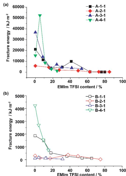
Fig. 2 Relationship between the fracture energy and ionic liquid (EMIm TFSI) content for (a) supramolecular ionic liquid elastomer (**A-Acrylate-1**) and (b) chemically cross-linked ionic liquid elastomer (**B-Acrylate-1**). [■: Methyl acrylate (1), ◆: ethyl acrylate (2), ▲: butyl acrylate (3), and ▼: methyl methacrylate (4)].
