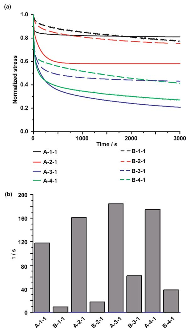
Fig. 3 (a) Stress relaxation behaviour of the supramolecular ionic liquid elastomer (**A-Acrylate-1**, solid lines) and chemically cross-linked ionic liquid elastomer (**B-Acrylate-1**, dashed lines) with a 5% strain for 1 hour. (b) Slow relaxation time constant of the **A-Acrylate-1** and **B-Acrylate-1**. Acrylate: methyl acrylate (1), ethyl acrylate (2), butyl acrylate (3), and methyl methacrylate (4).
