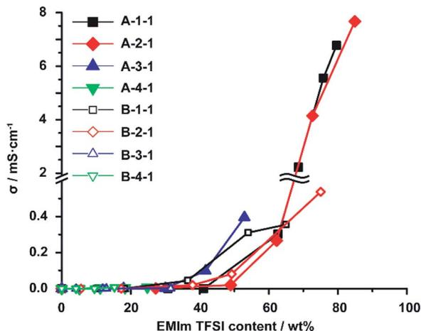
Fig. 4 Relationship between the ionic conductivity ( $\sigma$ ) and ionic liquid (EMIm TFSI) content for supramolecular ionic liquid elastomer (A-Acrylate-1) and chemically cross-linked ionic liquid elastomer (B-Acrylate-1). [■: Methyl acrylate (1), ◆: ethyl acrylate (2), ▲: butyl acrylate (3), and ▼: methyl methacrylate (4)].
