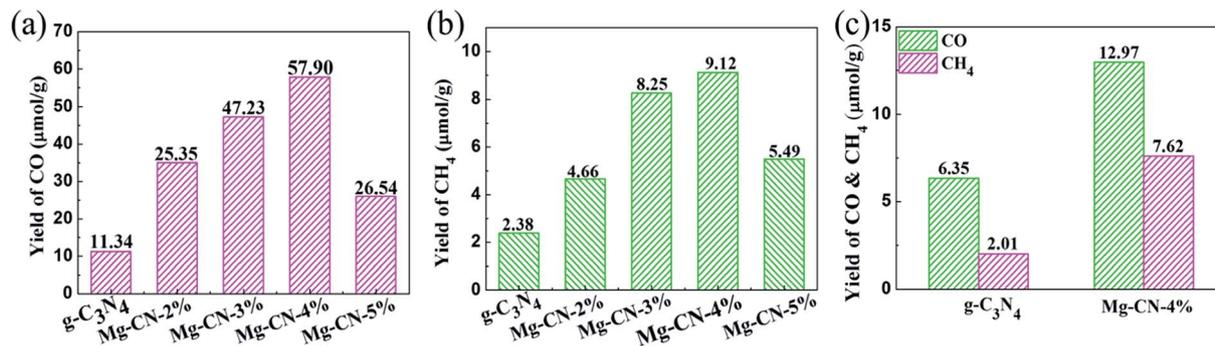
Fig. 5 UV-light photocatalytic activity of g-C<sub>3</sub>N<sub>4</sub> and Mg-doped g-C<sub>3</sub>N<sub>4</sub> samples (a) the yield of CO, (b) the yield of CH<sub>4</sub>; (c) visible-light activity of g-C<sub>3</sub>N<sub>4</sub> and Mg-CN-4%.
