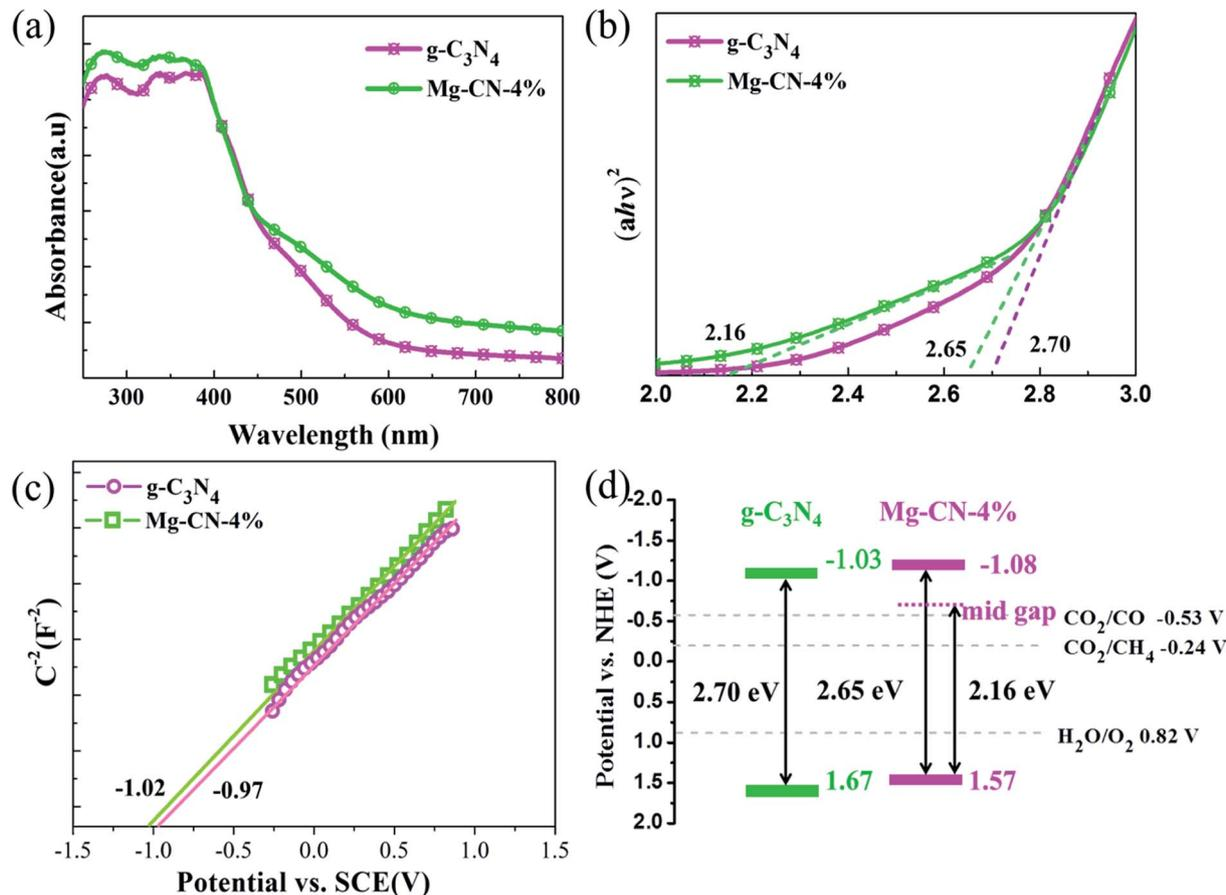
Fig. 3 (a) UV-vis diffuse reflectance spectra, (b) the plots of  $(ah\nu)^2$  versus  $h\nu$  for the band gap energies, (c) Mott-Schottky plots, (d) band gap structure of  $g\text{-C}_3\text{N}_4$  and Mg-CN-4%.
