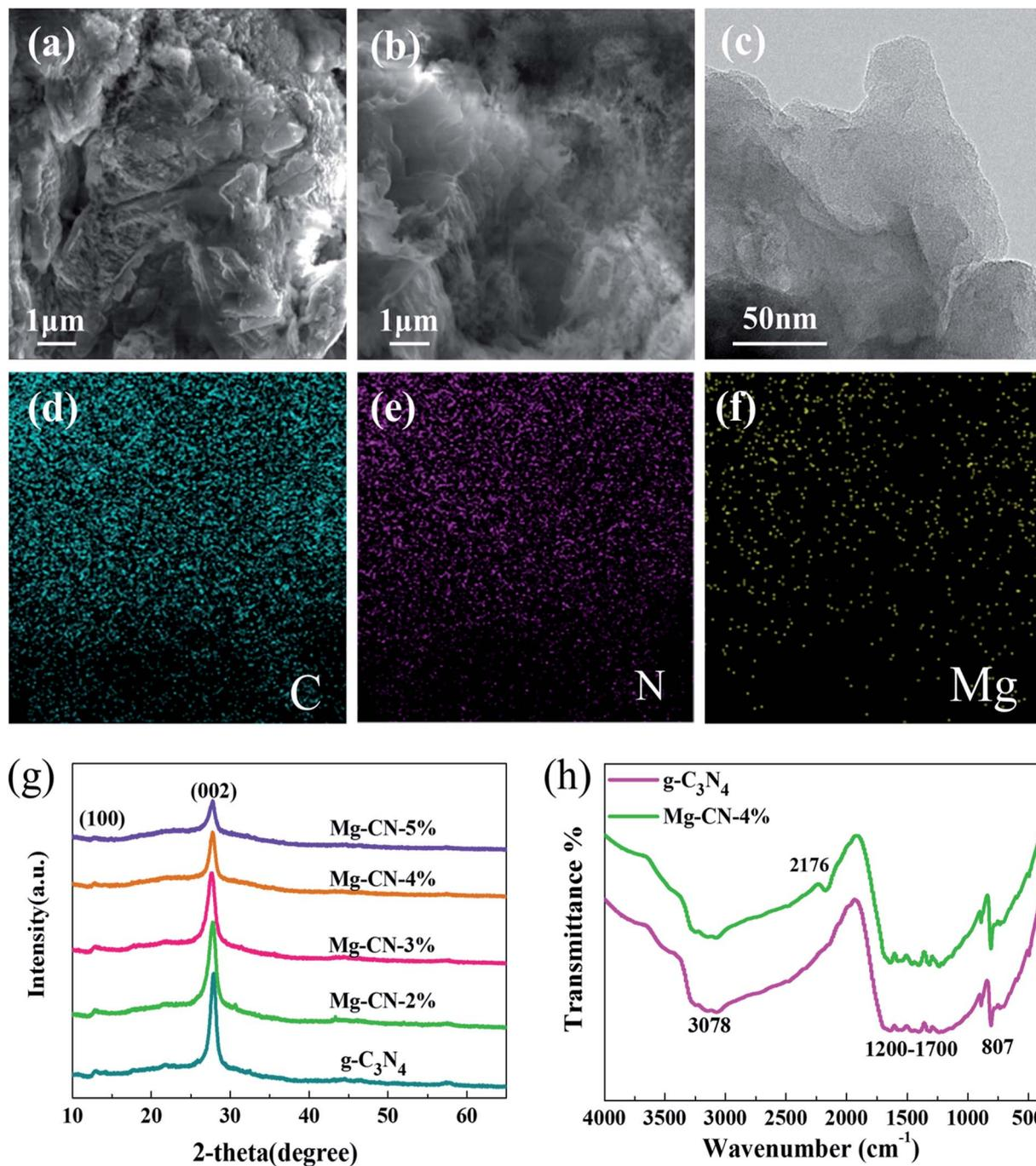
Fig. 1 SEM images of (a) g-C<sub>3</sub>N<sub>4</sub>, (b) Mg-CN-4%; (c) TEM image of Mg-CN-4%; (d) elemental mapping images of C, (e) N, (f) Mg of Mg-CN-4%; (g) XRD spectra of samples; (h) FTIR spectra of g-C<sub>3</sub>N<sub>4</sub> and Mg-CN-4%.
