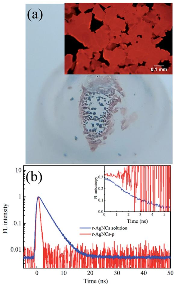
**Fig. 3** (a) The r-AgNCs-p under ambient light. The inset shows the FL microscope image of the r-AgNCs-p. (b) The FL decay dynamics ( $\lambda_{\text{ex}}/\lambda_{\text{em}} = 580 \text{ nm}/640 \text{ nm}$ ) of the r-AgNCs-p and the r-AgNCs solution. The inset indicates the corresponding FL anisotropy dynamics probed at the same wavelength.
